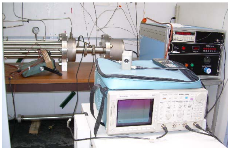
Figure 4. \text{H}_2 switch reactor with oscilloscope.
