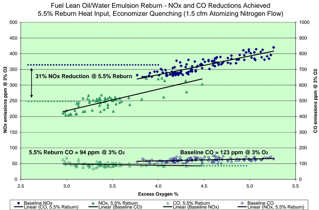
**Figure 8. Fuel Oil/Water Emulsion Reburn Results at 5.5% Reburn Fuel Heat Input**
