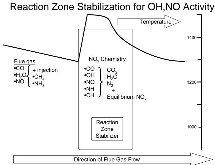
**Figure 10. A Schematic Representation of Reaction Zone Stabilizer Chemistry**
