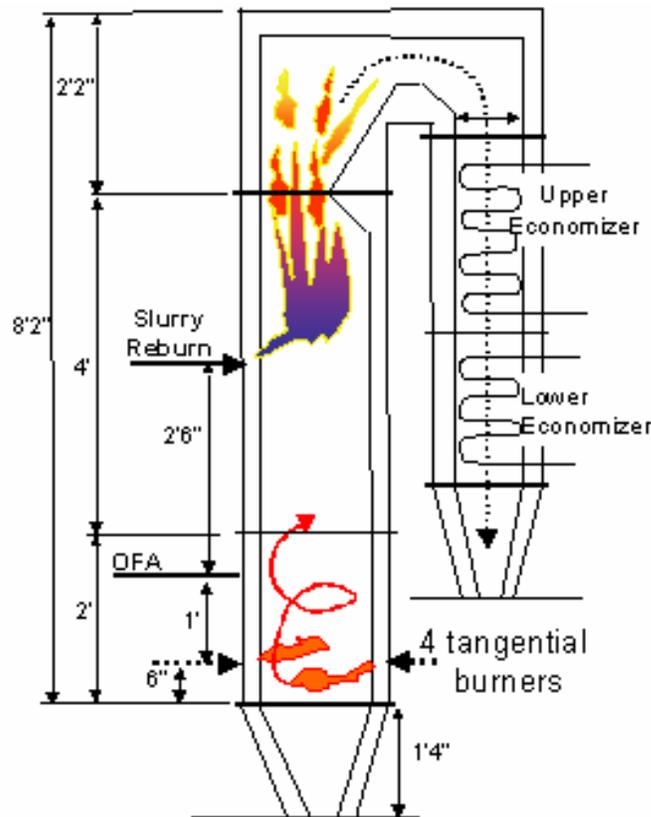
**Figure 5. Reburn Fuel Injection Location**
