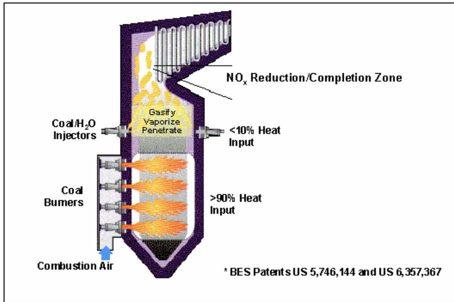
Figure 1 Coal/Water Slurry Reburn Process Schematic
