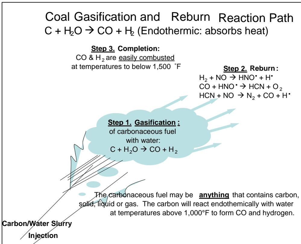
Figure 2. Coal Gasification and Reburn Reaction Path
