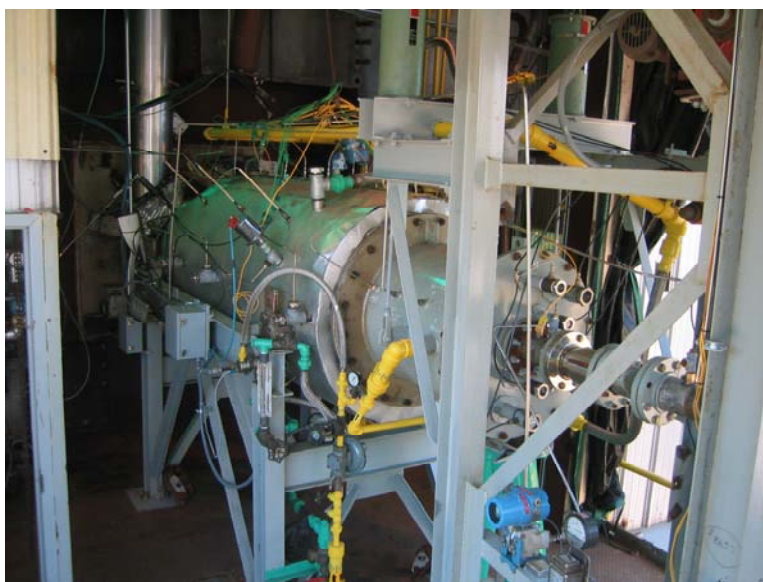
Figure 4. Large-scale prototype coal preheating combustor installed in the CBTF at Riley Power Inc's R&D Center
