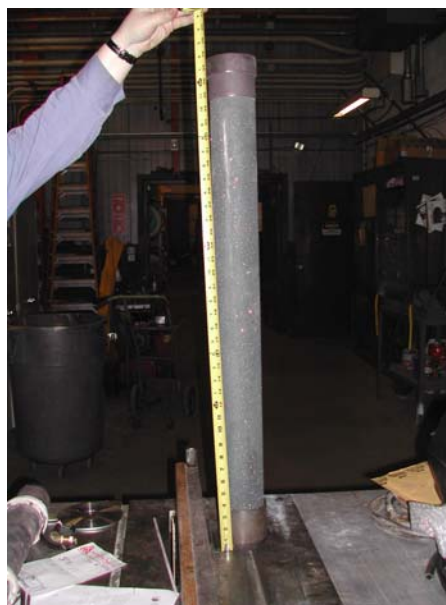
Figure 3. Silicon carbide indirect air-cooled liner with transition pieces
