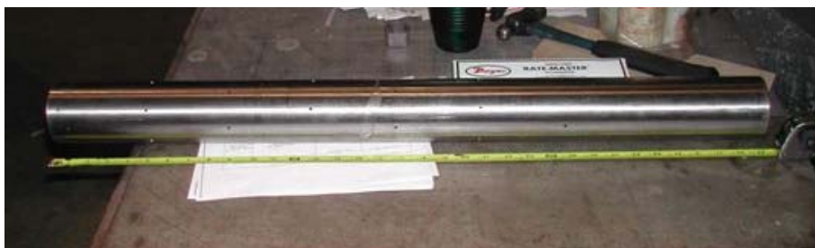
Figure 1. Air-bleed stainless steel liner with 54 1/8-in diameter holes prior to attachment of transition pieces.
