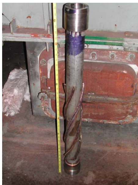
Figure 2. Stainless steel indirect air-cooled liner with spiral fins and transition pieces
