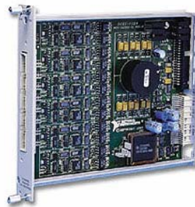
Figure 17 - 1124- Analog Output Module
