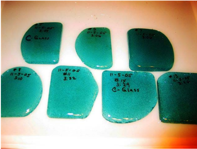
Figure 13. C-glass patties collected during 11-5-05 melting trial
