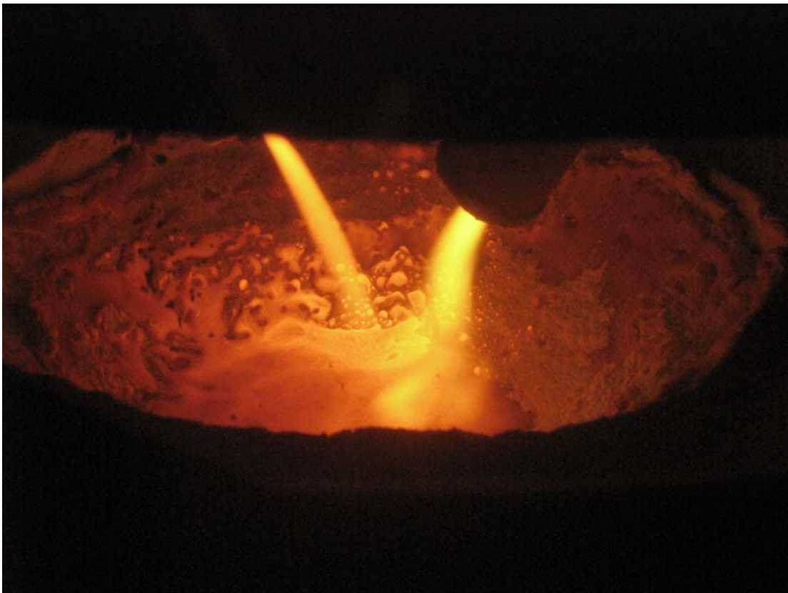
Figure 2. Plasma Torches in S-Glass Melting Operation
