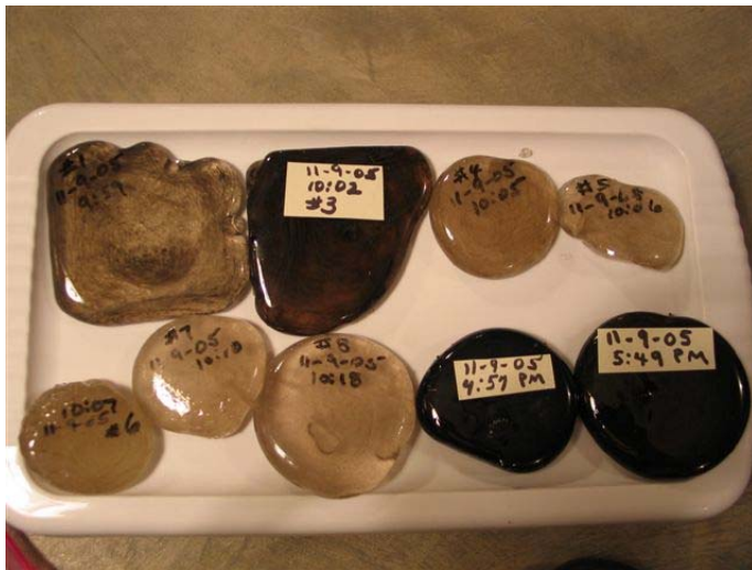
Figure 20. Suite of Low DK Glass patties produced during the plasma melting trial
