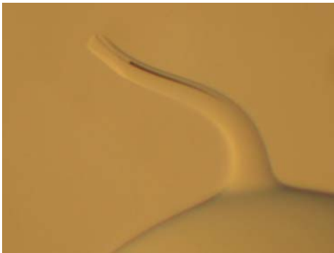
Figures 8a & 8b. Dark Lines In Fiber Tips Are Hollow Filaments (seeds/bubbles) That Likely Caused The Fiber to Break Out
