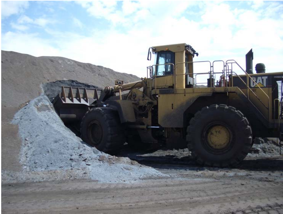
Figure 18. The excavation of the steel slag stockpile to provide materials for pilot testing.
