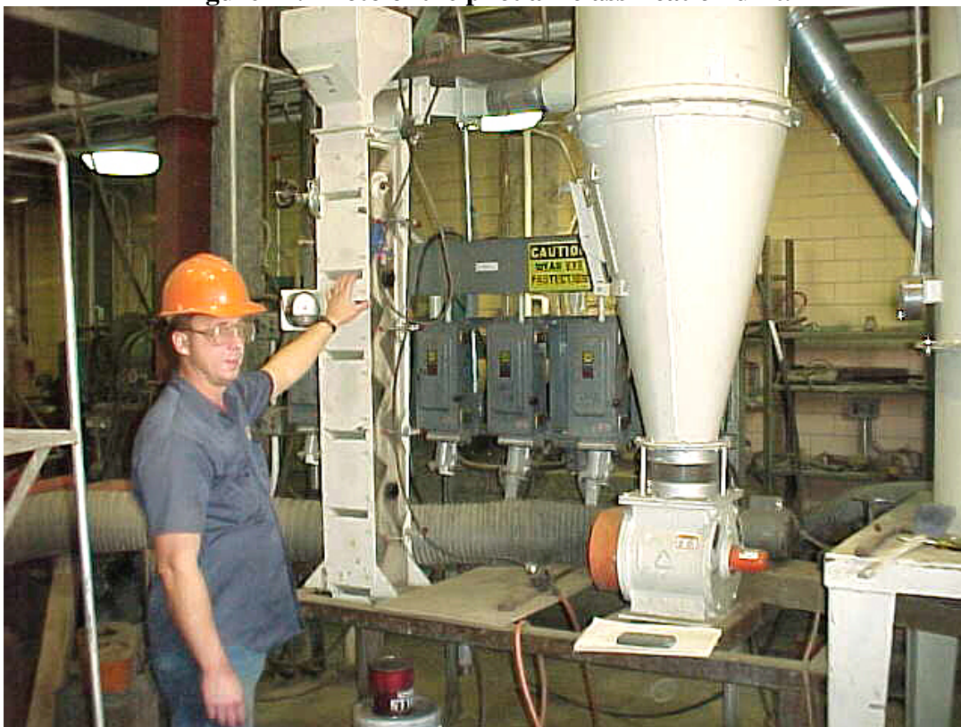
Figure 17. Photo of the pilot air classification unit.
