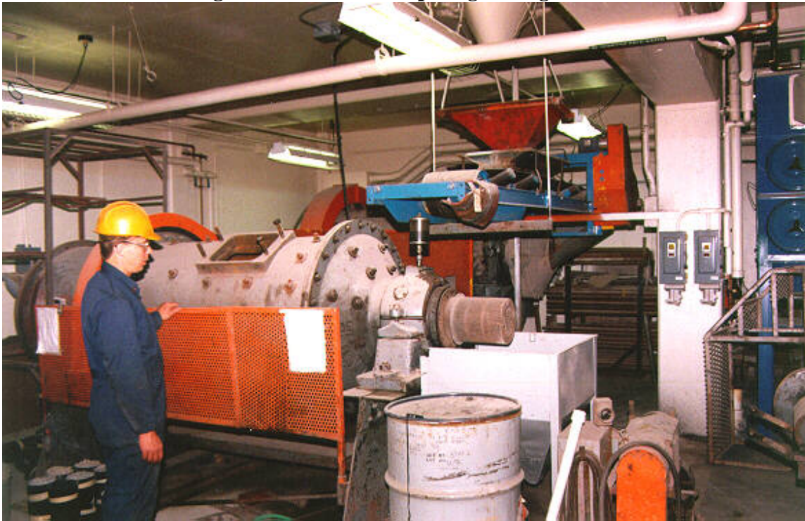
Figure 16. Photo of the pilot grinding circuit.
