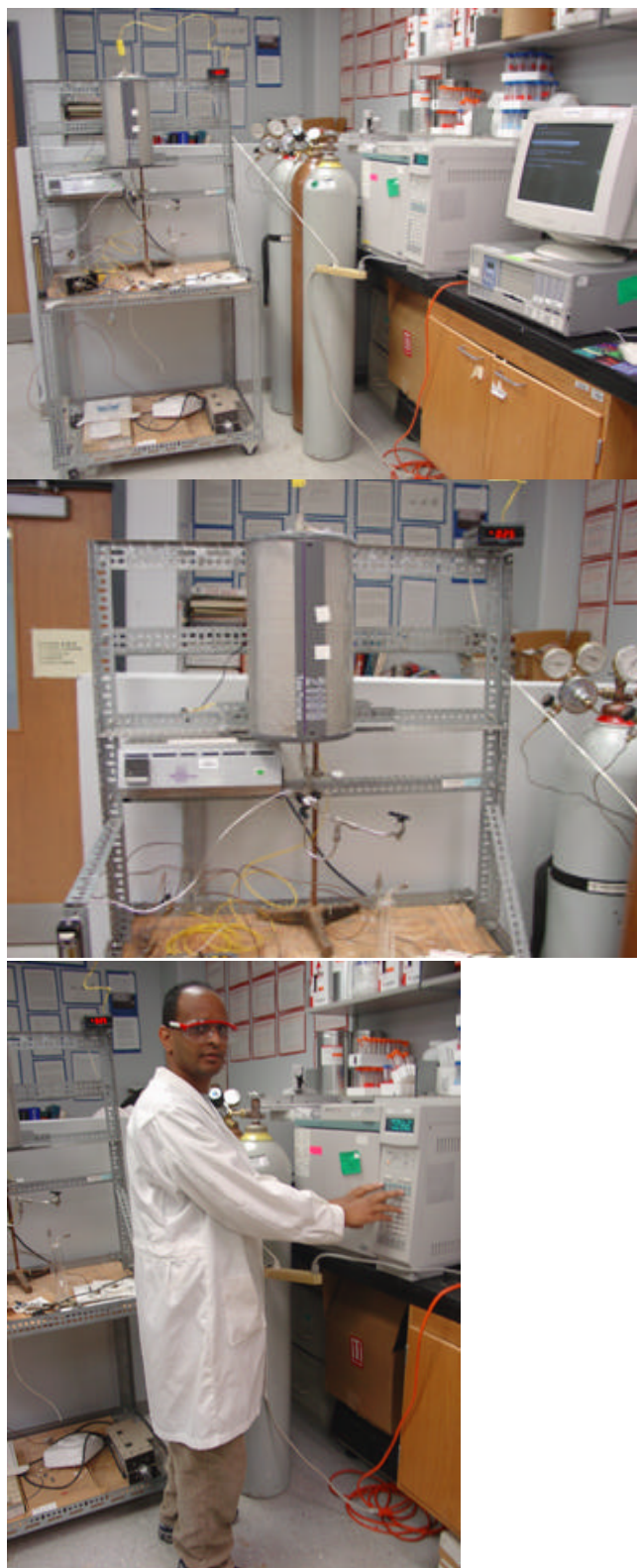
Figure 1. Pictorial of the single pass fixed bed continuous flow reactor catalytic reactor interfaced with for evaluating cumene cracking
