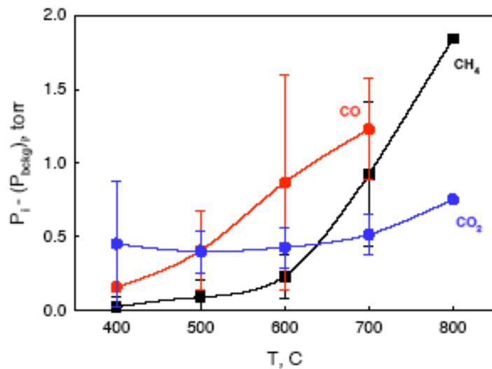
Figure 9: Total pressure dependence with temperature for EBS decomposition.
