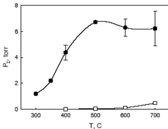
Figure 6: Temperature dependence of total pressure measured after 1 h of heating and corrected for background of CO and CO<sub>2</sub> from the Fe-C mixture.
