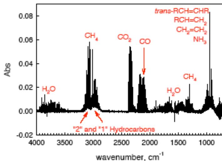
Figure 7: IR spectra of the gas-phase products measured at 700°C.
