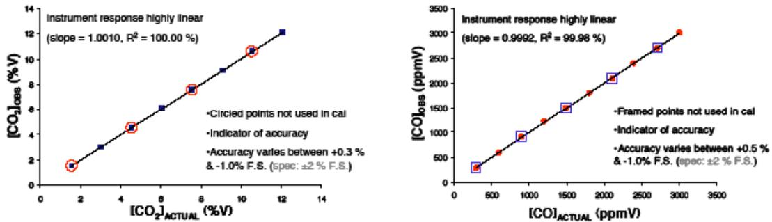
Figure 12: Performance data using breadboard analyzer.
