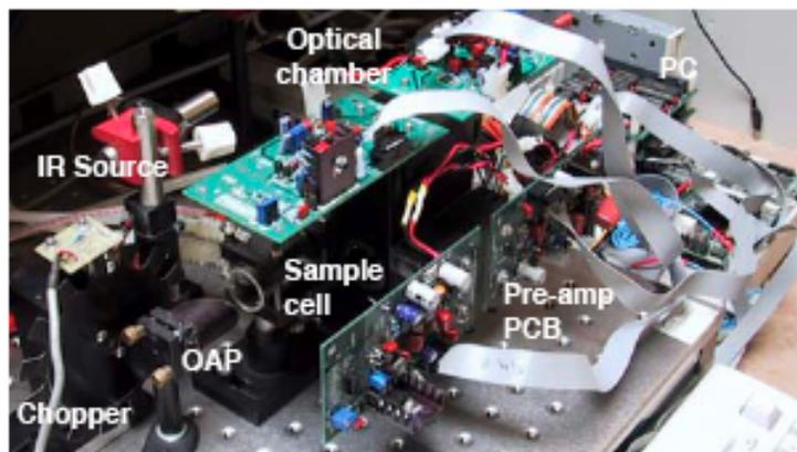
Figure 10: Breadboard gas analyzer.
