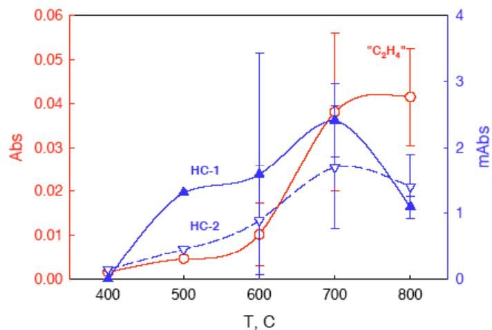
Figure 8: Temperature dependence of absorbance corresponding to hydrocarbon chains.
