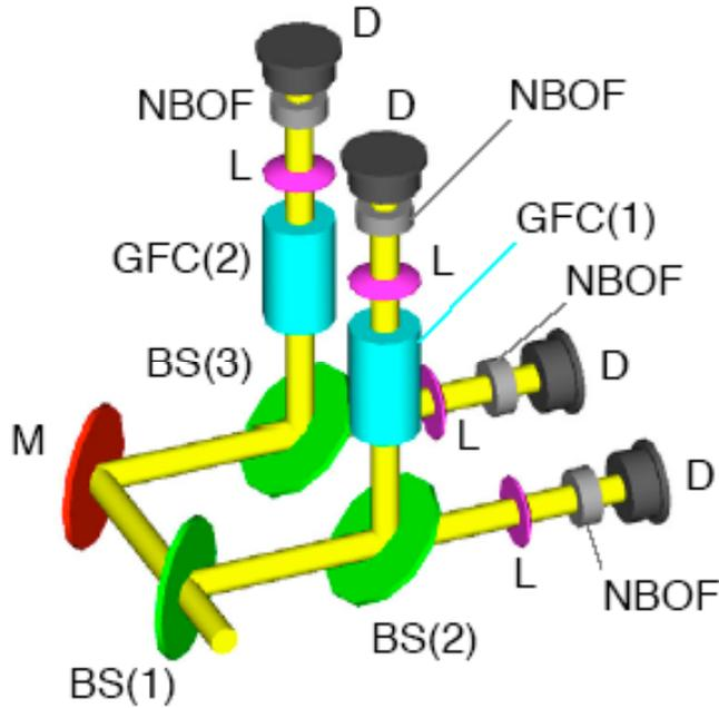
Figure 11: Schematic diagram showing the operational principle of the breadboard gas analyzer.
