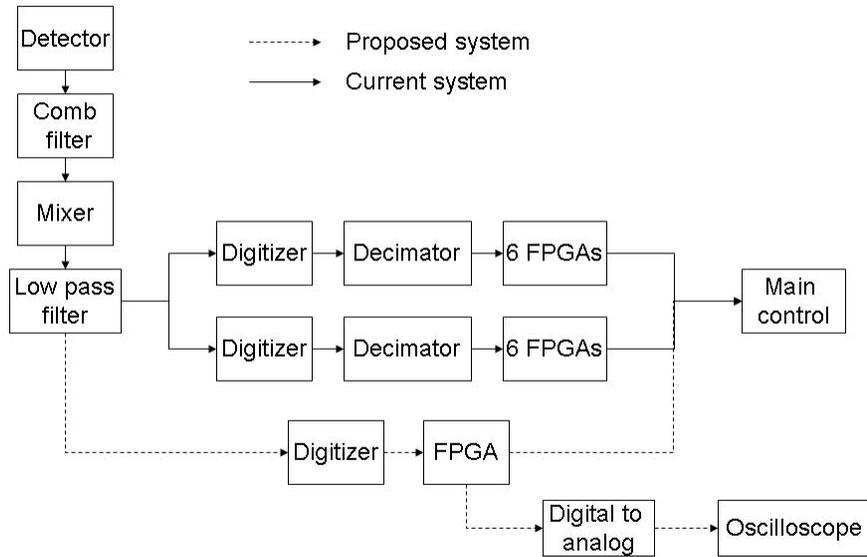
Figure 1: A diagram comparing the old system to the proposed system. The proposed system replaces 6 FPGAs with one and does not need a decimator.
