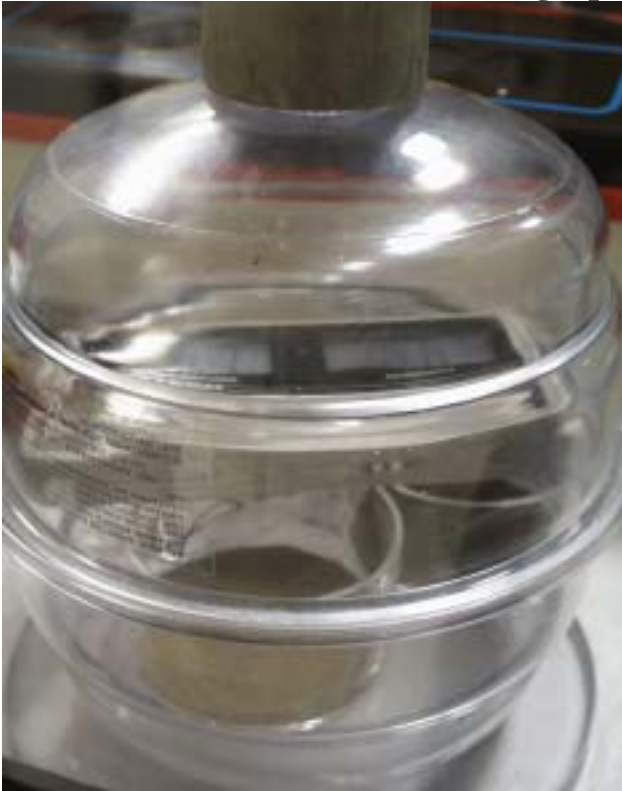
Figure 11. Exposure of NpO 2 to 75% RH prior to test 1.
