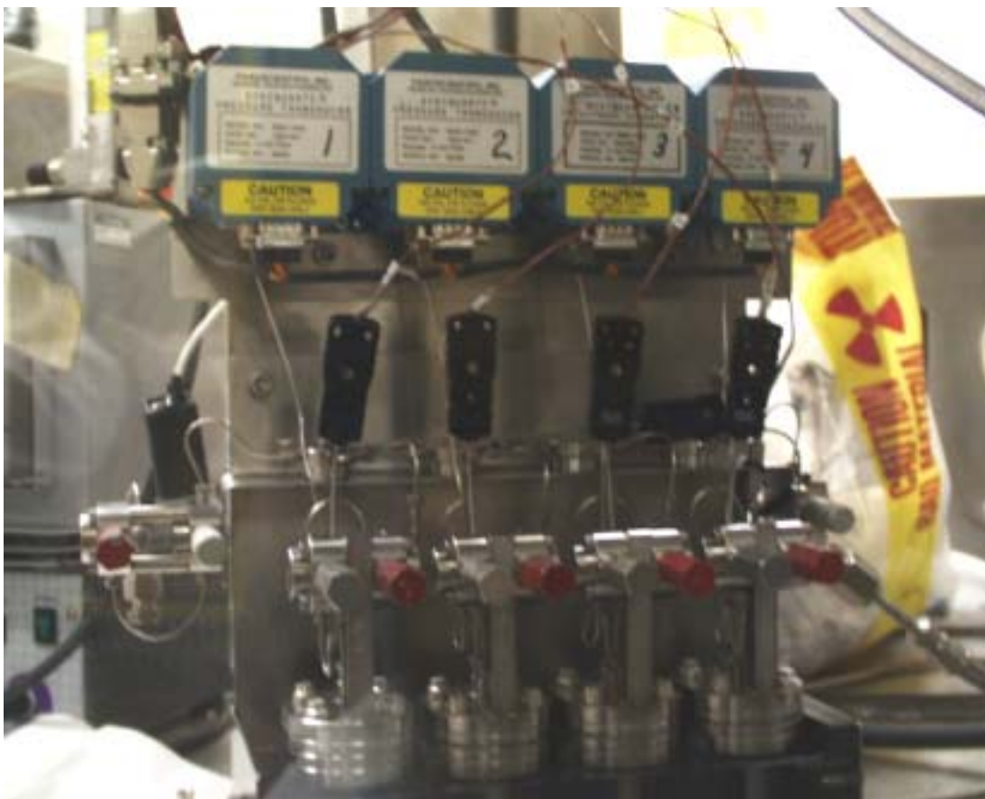
Figure 4. Photograph of test vessels loaded with \text{NpO}_2 .
