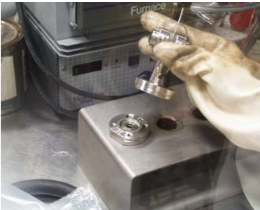
Figure 14. Installing test vessel top for \text{NpO}_2 gas generation test.
