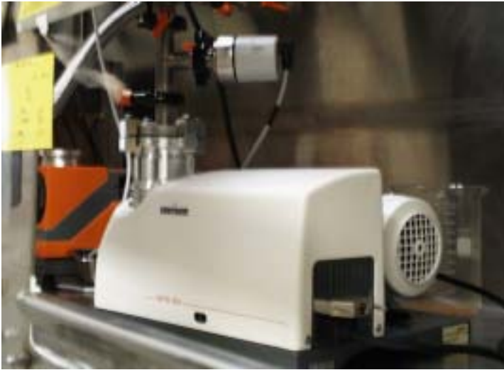
Figure 17. Alcatel Drytel Model 1025 vacuum pump installed in radioactive containment.
