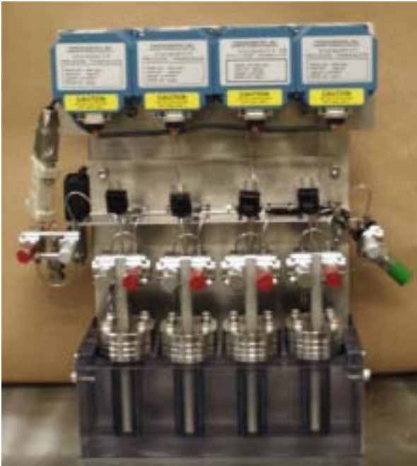
Figure 15. Test apparatus for NpO 2 gas generation experiments.
