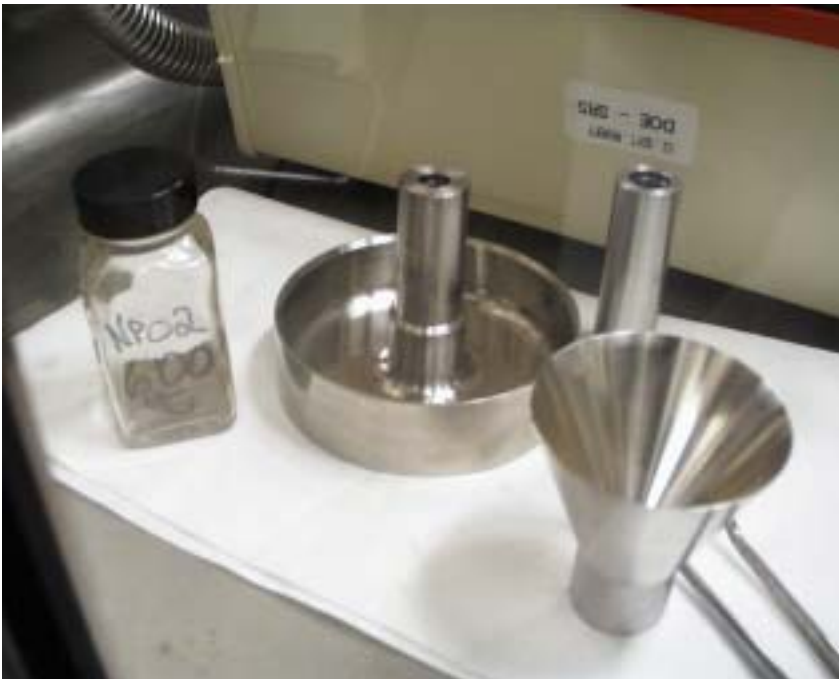
Figure 12. Equipment used in loading test vessel inserts.
