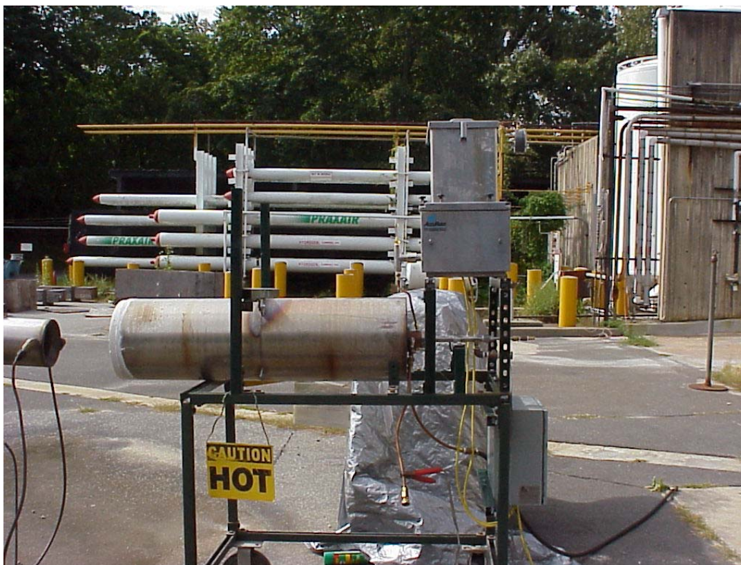
Figure 4-18. Photograph of hot oxygen test rig
