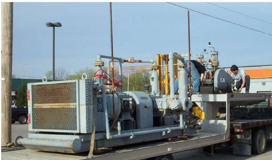
Figure 1 Ariel compressor as removed from City site.
