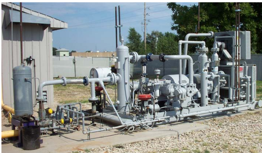
Figure 2. Ariel JG/2 compressor as installed at NGML.
