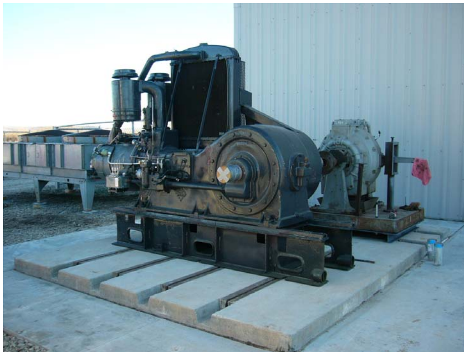
Figure 4 Ajax Engine and Dynamometer.
