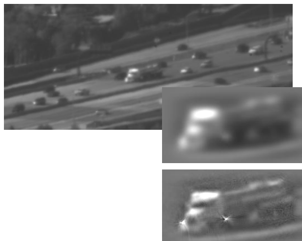
Figure 1: Before and after speckle processing of a semi-truck at 13 km range traveling at highway speeds.
