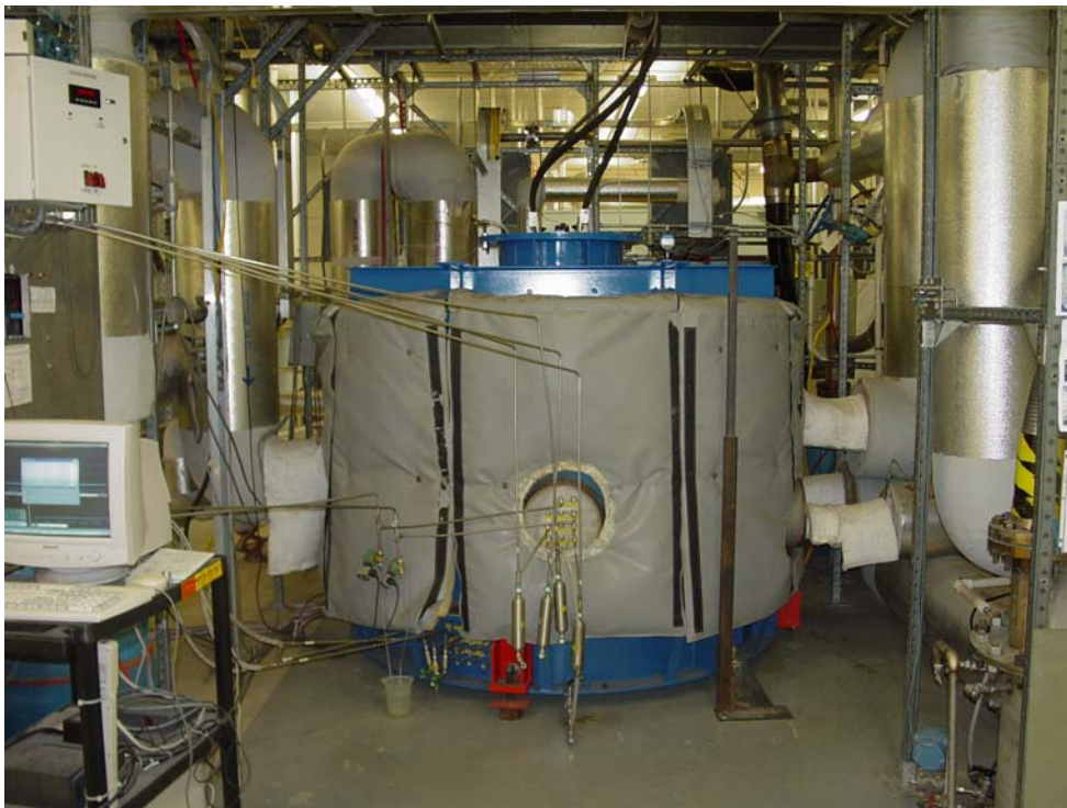
Figure 4. 20 kW STACK USED FOR TESTS OF CASCADED FUEL CELL CONCEPT:
