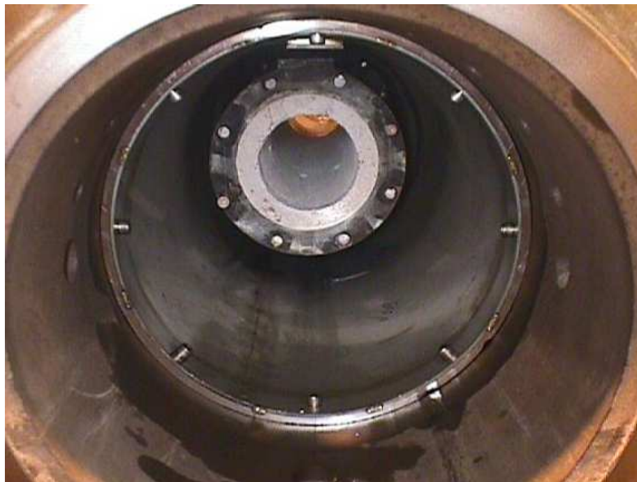
Figure 3-30 Ceramic combustion liner inside of test vessel
