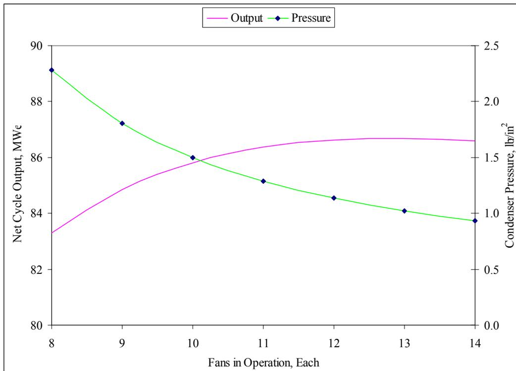
Figure 9 Plant Performance and Air Cooled Condenser Operation
