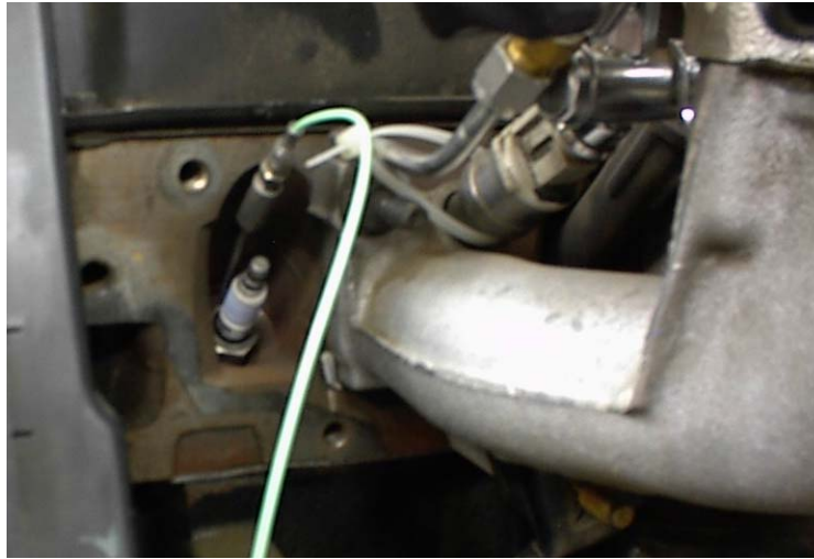
Figure 14. Modified spark plug with pressure transducer installed.
