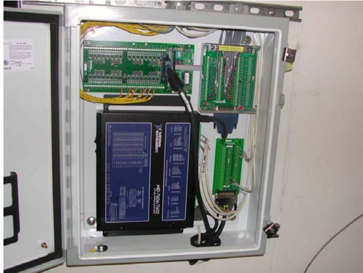
Figure 11. Main panel for data acquisition and control equipment. Top left AMUX-64T, top right SCB-68, bottom left MID-7604, bottom right CB68-LPR
