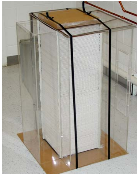
Figure 7.2. EERV core assembly for demonstrator unit.
