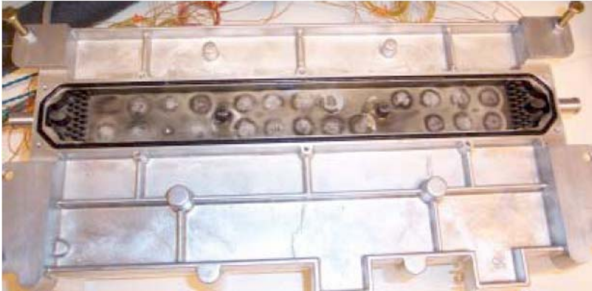
Fig. 1. Photograph of a modified Semikron heat sink.
