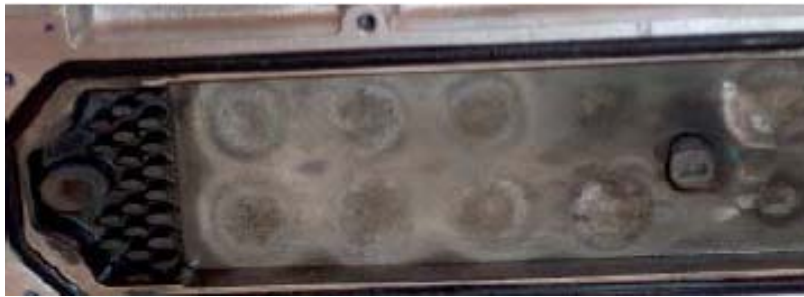
Fig. 7. Photograph of heat-sink corrosion.
