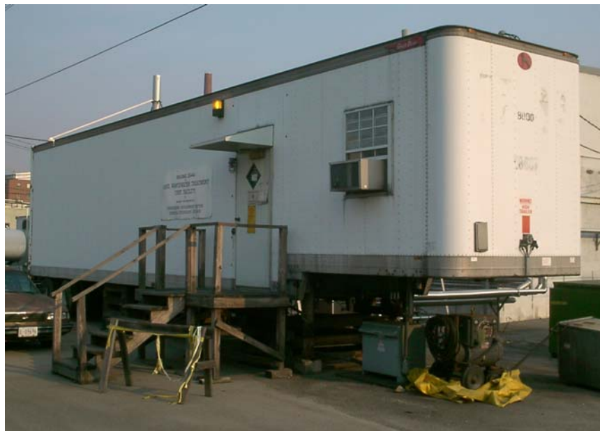
Fig. 6.1. Long term testing of surrogate sludge was conducted under ambient conditions within an unconditioned section of OR trailer. Samples were subjected to natural extremes of temperature and humidity over the course of 9 months.
