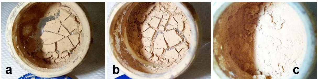
Fig. 3.10. (a) Dried MVST W24 sample – no additives, (b) Dried MVST W25 sample – no additives, (c) Dried MVST W28 sample – No additives. Note powdery appearance.
