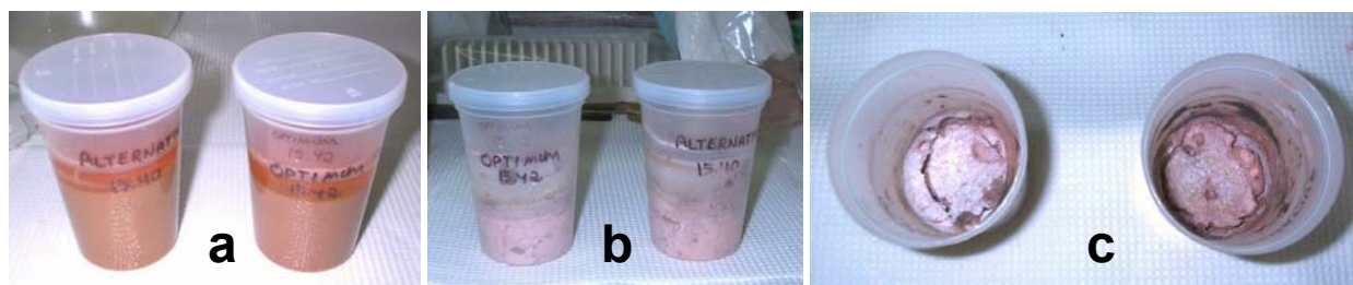
Fig. 3.2. (a) Rinsed QnD sludge after FWENC additives, before drying, (b) Rinsed QnD sludge after FWENC additives, after drying, and (c) Rinsed QnD sludge after FWENC additives, after drying, top view
