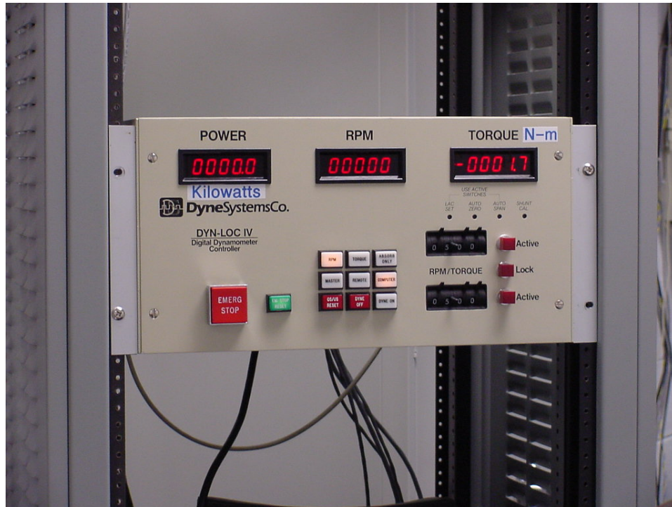
Fig. 3. Dynamometer controller display panel.
