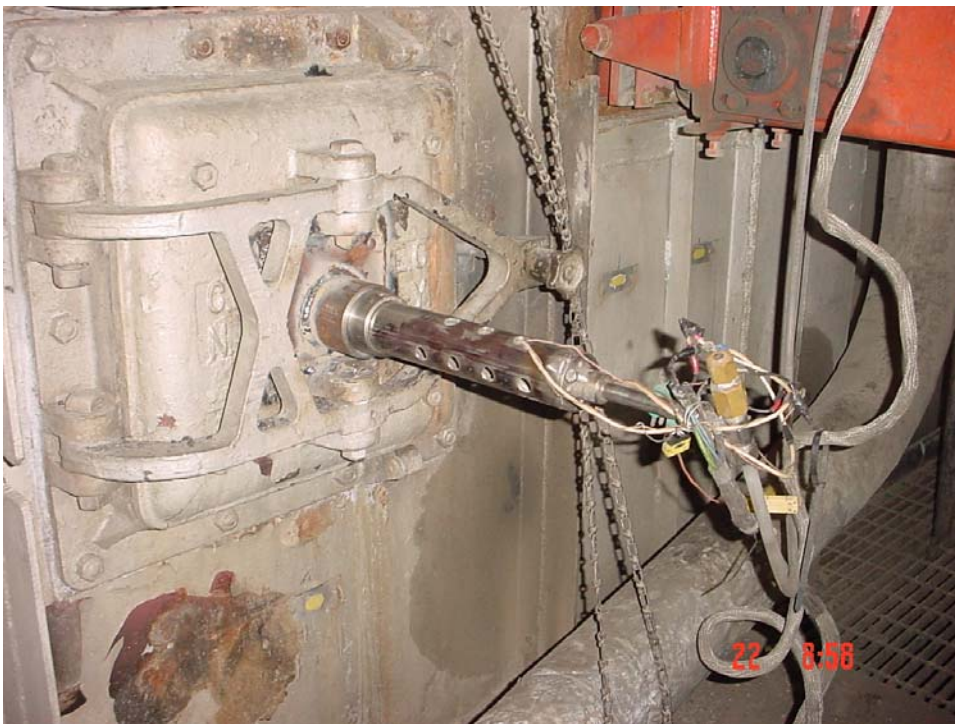
Figure 14 Corrosion probe inserted through the manhole at superheaters.
