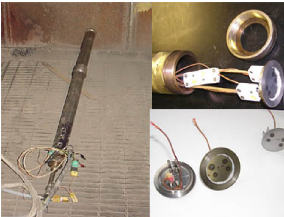
Figure 12 Corrosion probe (left) and the sensor assembly (right)
