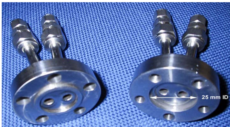
Figure 6. New stainless steel flow cell for 25 mm diameter membrane samples.
