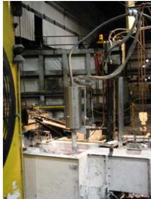
Figure 21 - LIBS Probe Installed at Commonwealth
