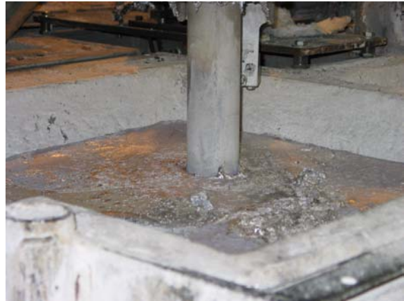
Figure 21 - LIBS Probe Installed at Commonwealth
