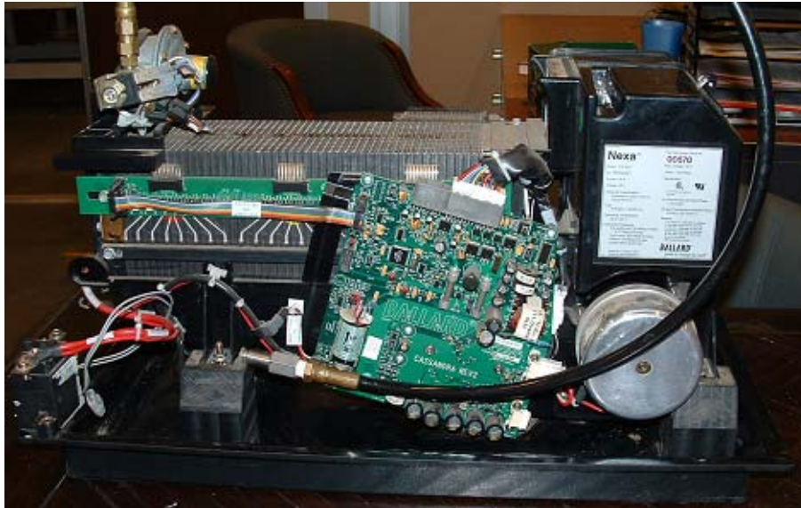
Figure 8: 1.2 kW NEXA Fuel Cell Power Module
