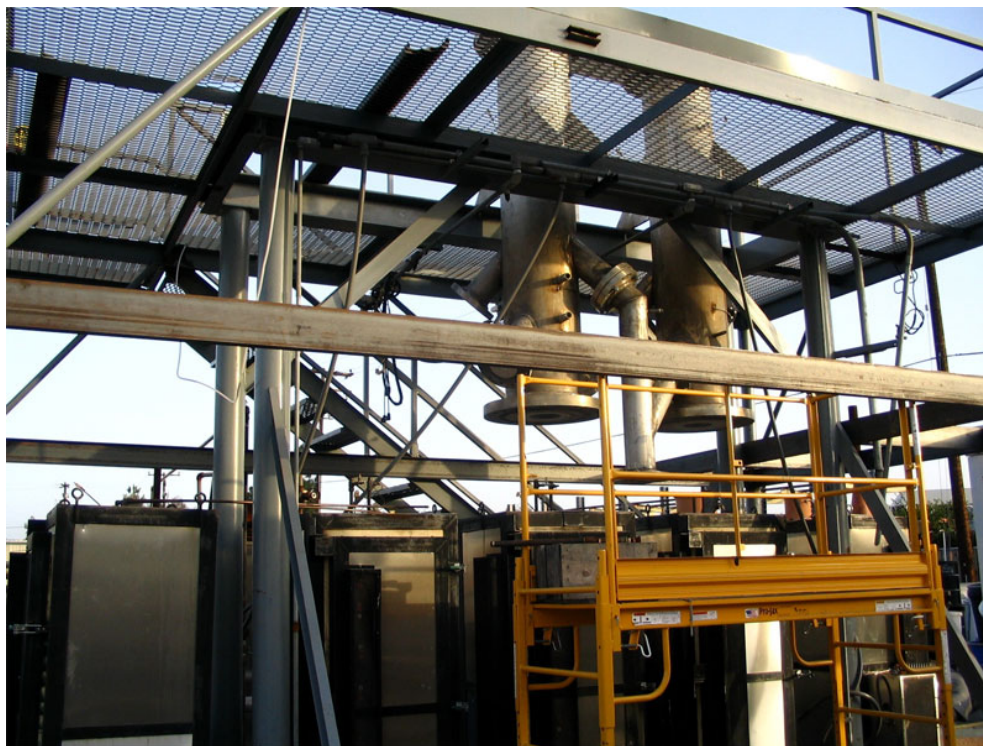
Figure 2-16 Photo of reactors shown assembled on support frame—bottom view
