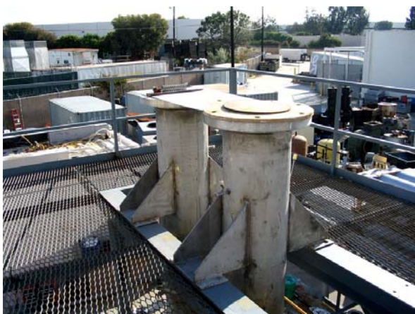
Figure 2-15 Photo of reactors shown assembled on support frame--top view
