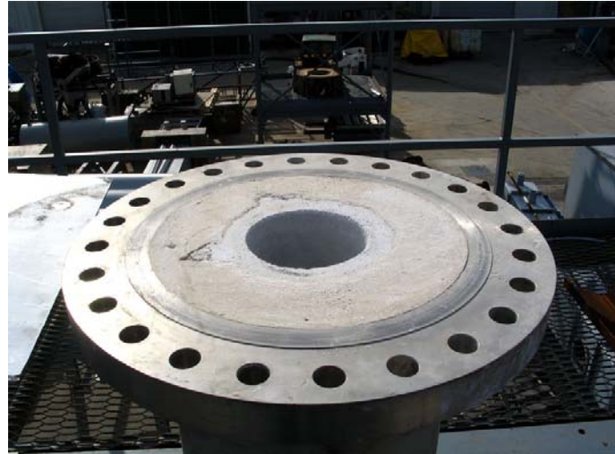
Figure 2-13 Photo of Reactor 1 refractory layers.
