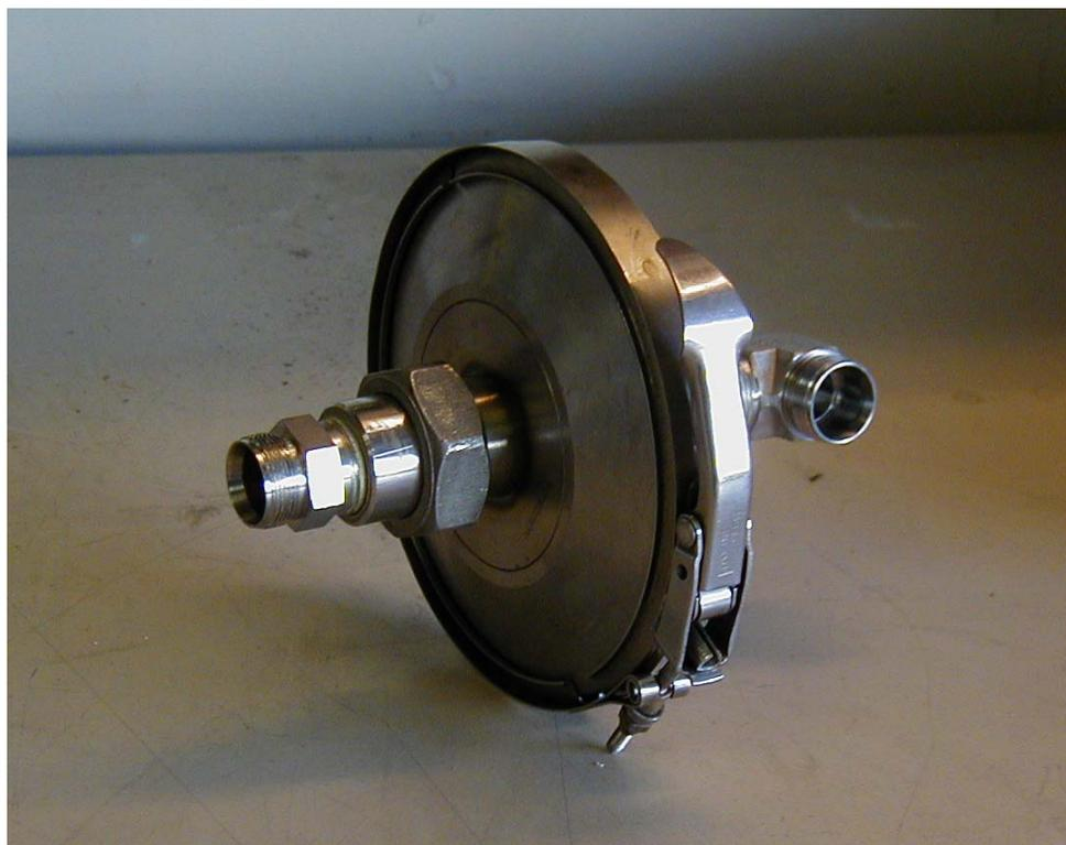
**Figure 2-2. Particulate Matter Filter Holder**
