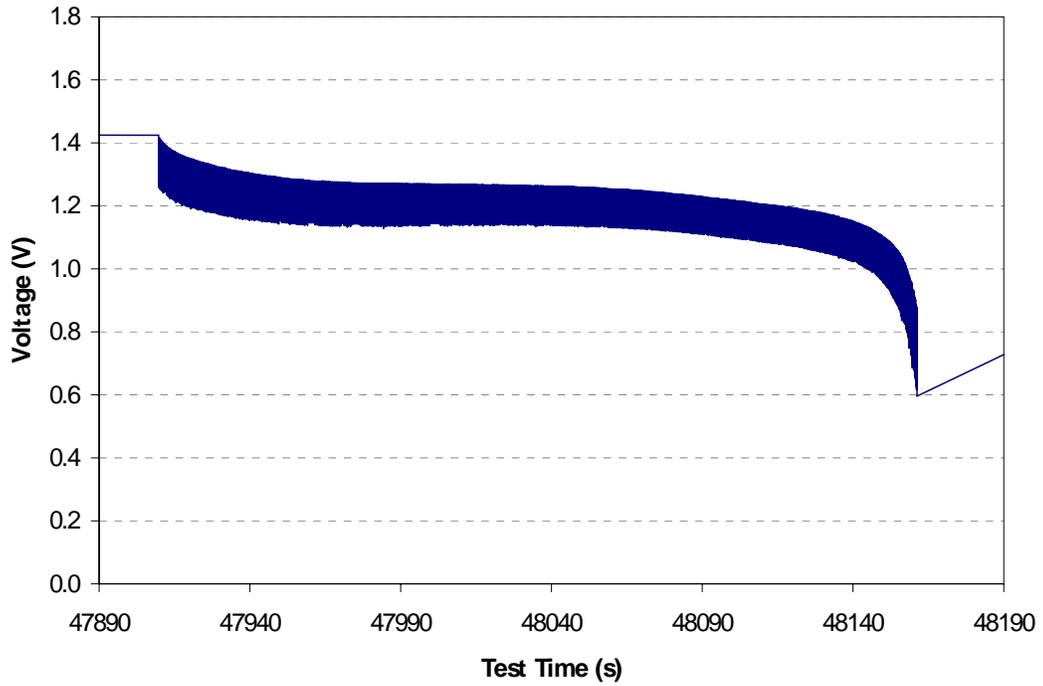
**Figure 14: Pulse discharge of cell S121-3 starting at 100% SOC**
