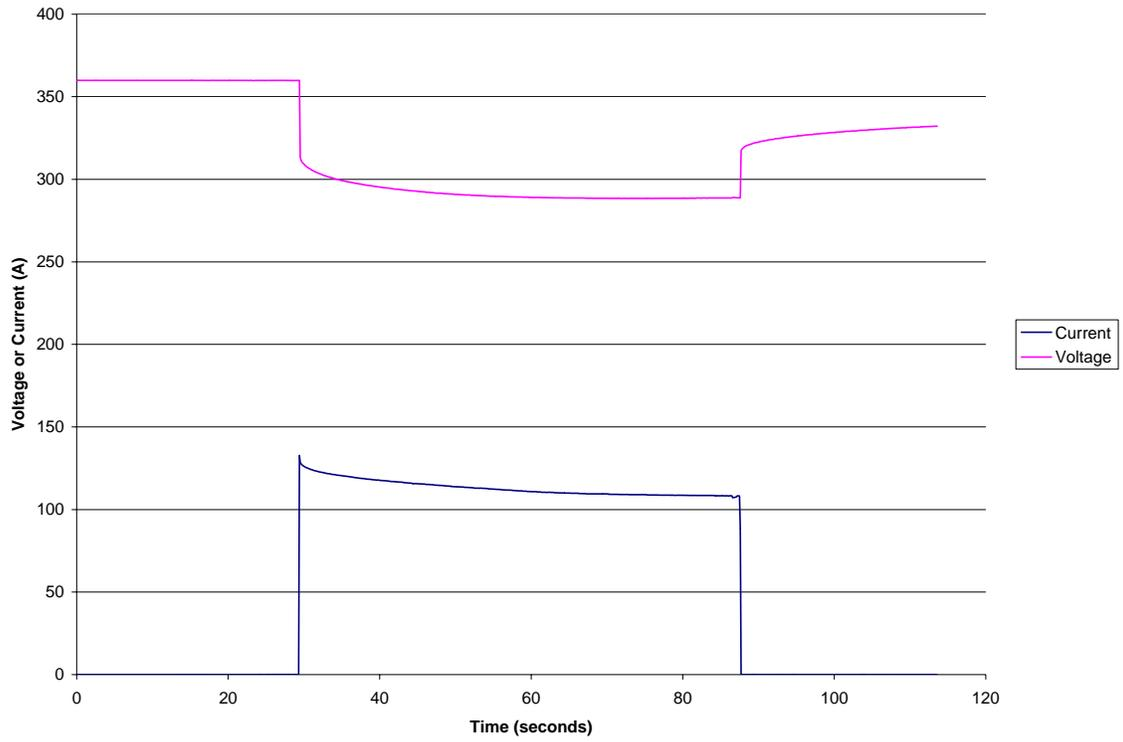
**Figure 59: Low rate discharge at average I = 3.86A. Capacity = 3.25Ah**
