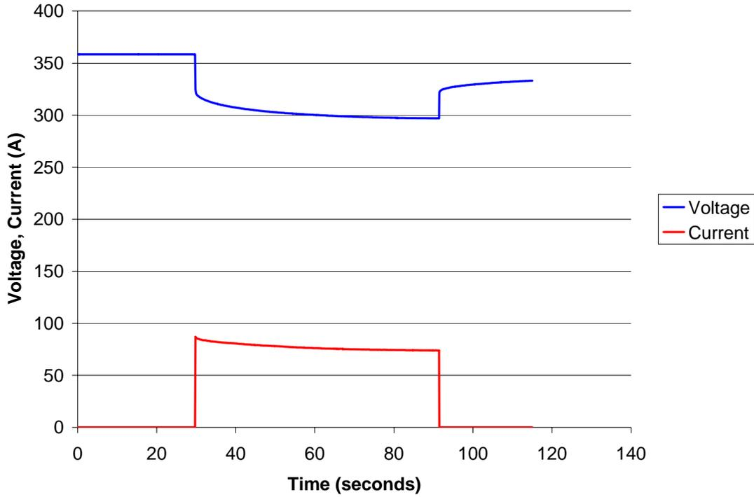
**Figure 55: Low current discharge ( $I_{avg} = 3.25A$ ). Capacity removed = 3.76Ah**
