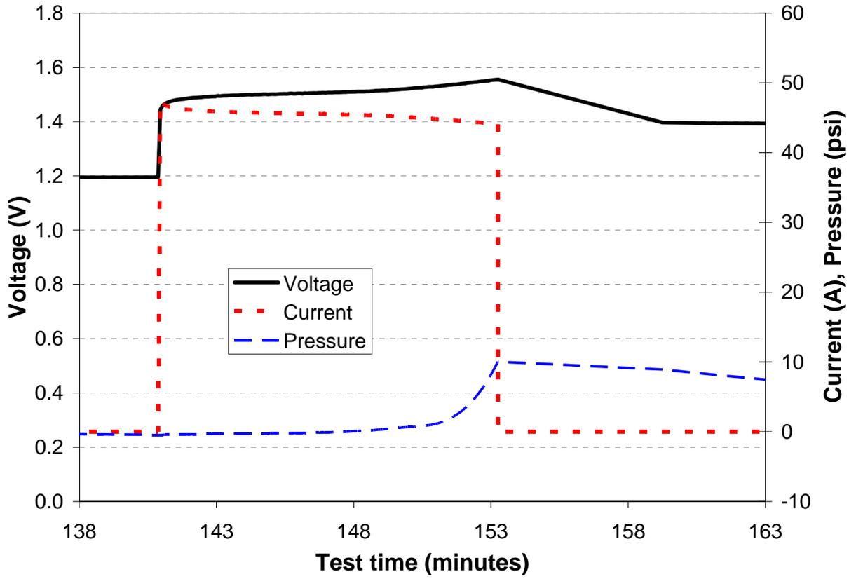
**Figure 20: PEDV Discharge Test 12.96 Ah**
