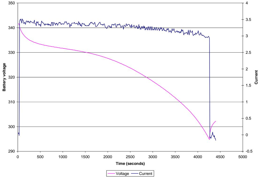
**Figure 44: Battery recharge at 2A. Capacity input = 4.85Ah total**
