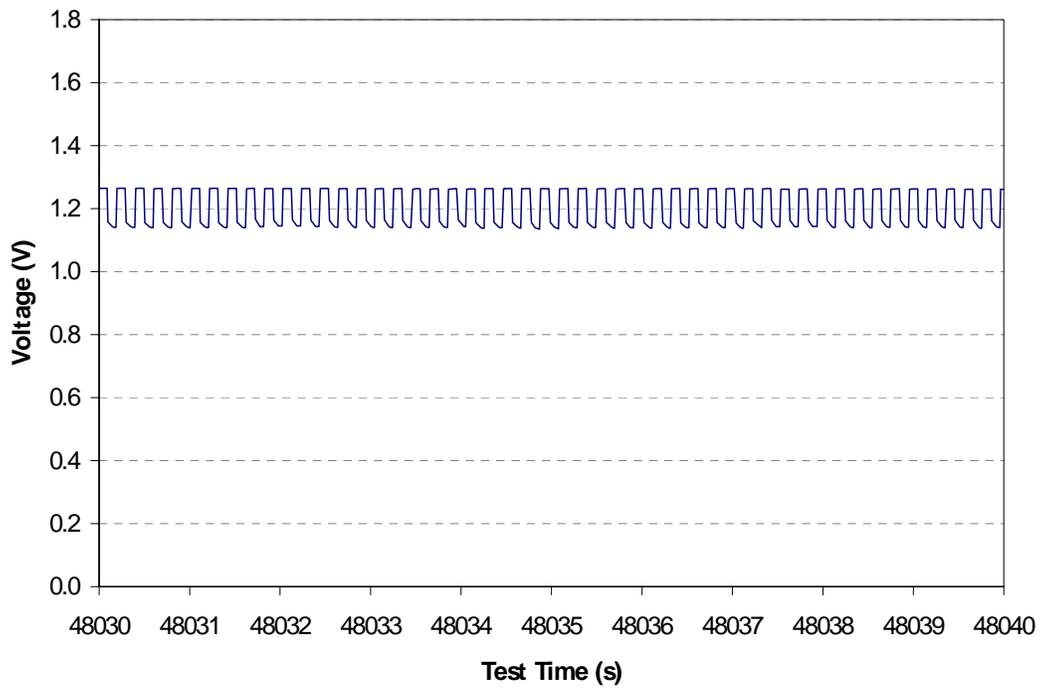
**Figure 15: Pulse discharge of cell S121-3 starting at 100% SOC**
