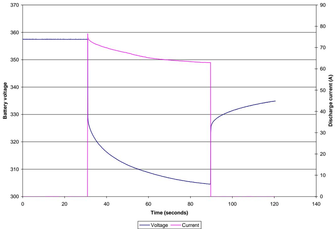
**Figure 37: Rest data after 1<sup>st</sup> high current discharge**
