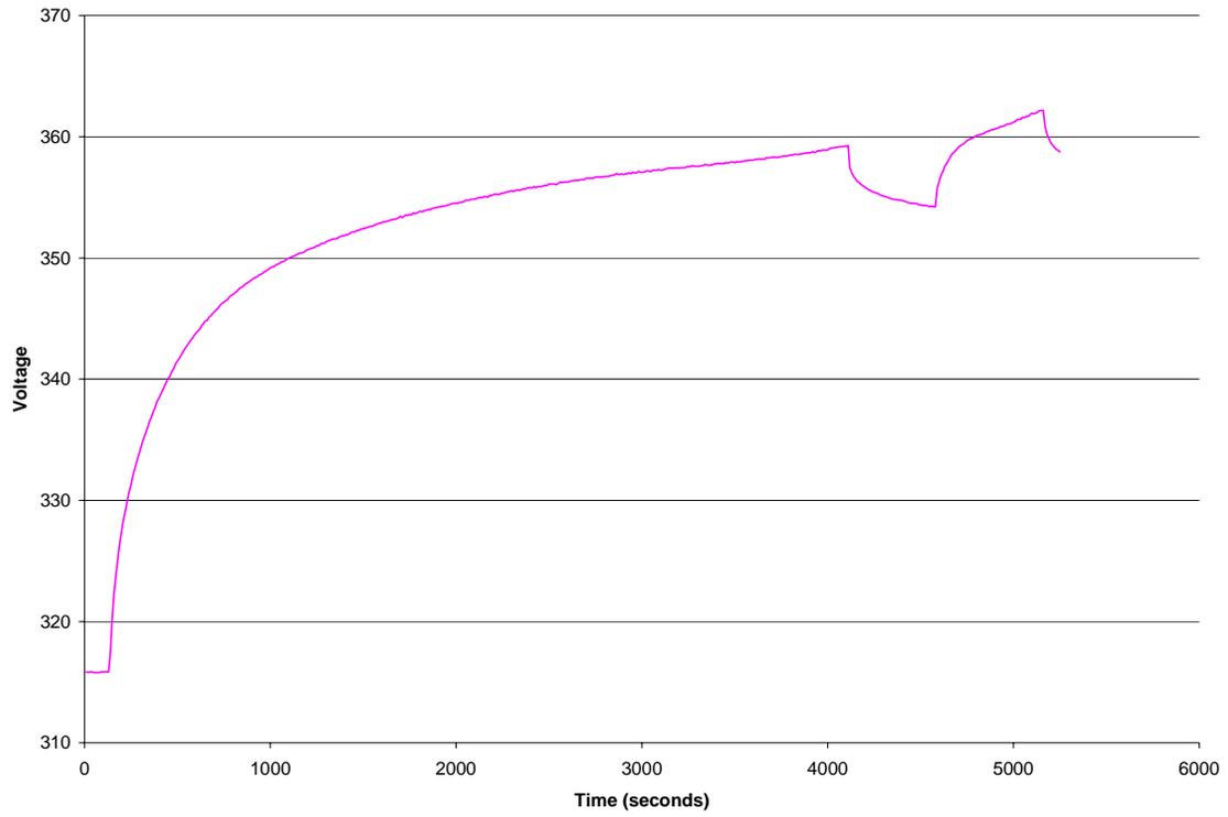
**Figure 61: Discharge at average current of 124.0A for 10.6 seconds**
