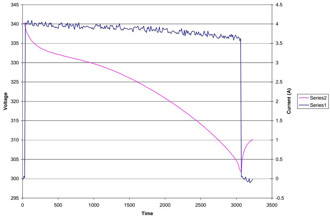
**Figure 60: Recharge at 2A. Charge capacity = 2.52Ah**
