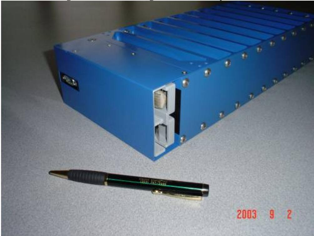
**Figure 25: High-Power Battery Module with Control Box**
