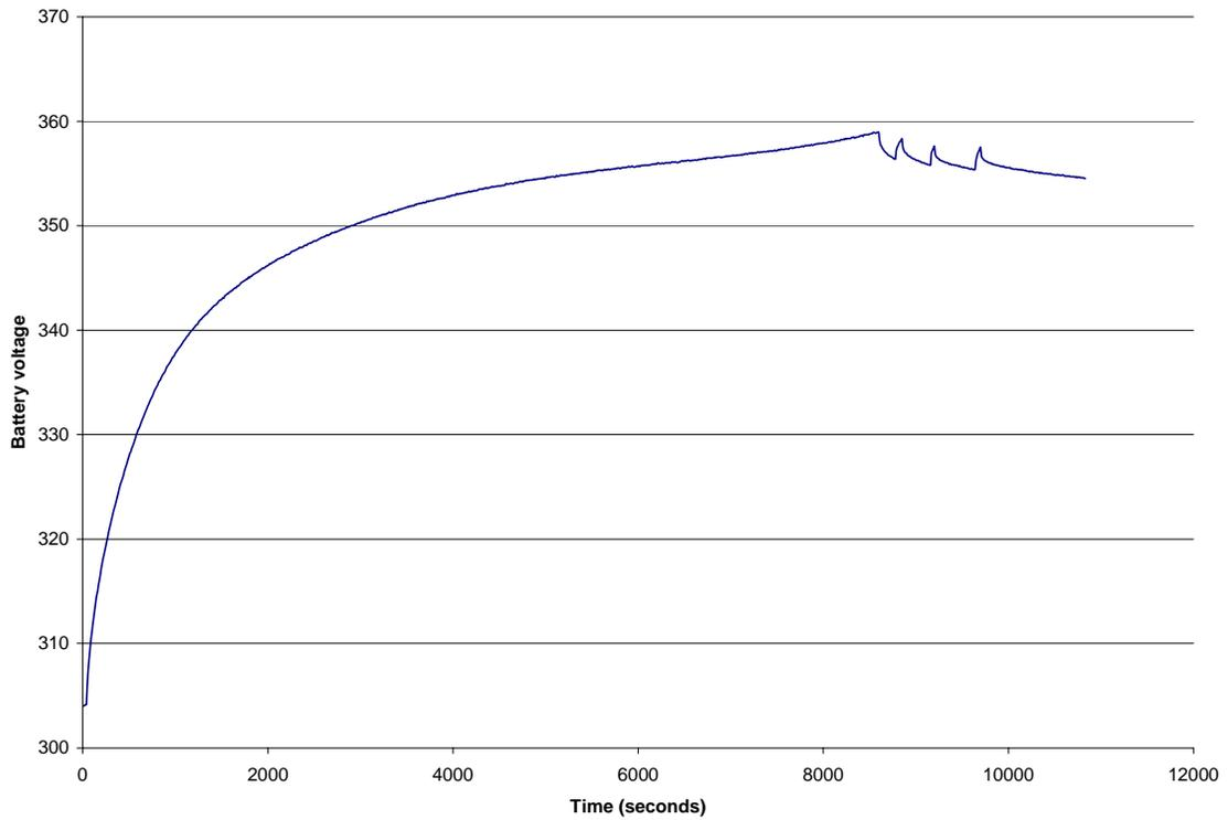
**Figure 45: Continuation of charge after overnight stand. Charge input = 0.80Ah.**
