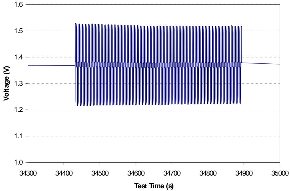
**Figure 12: Pulse cycling of cell S121-3 at 50% SOC**
