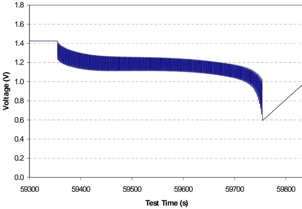
**Figure 16: Pulse discharge of cell S121-3 starting at 100% SOC**
