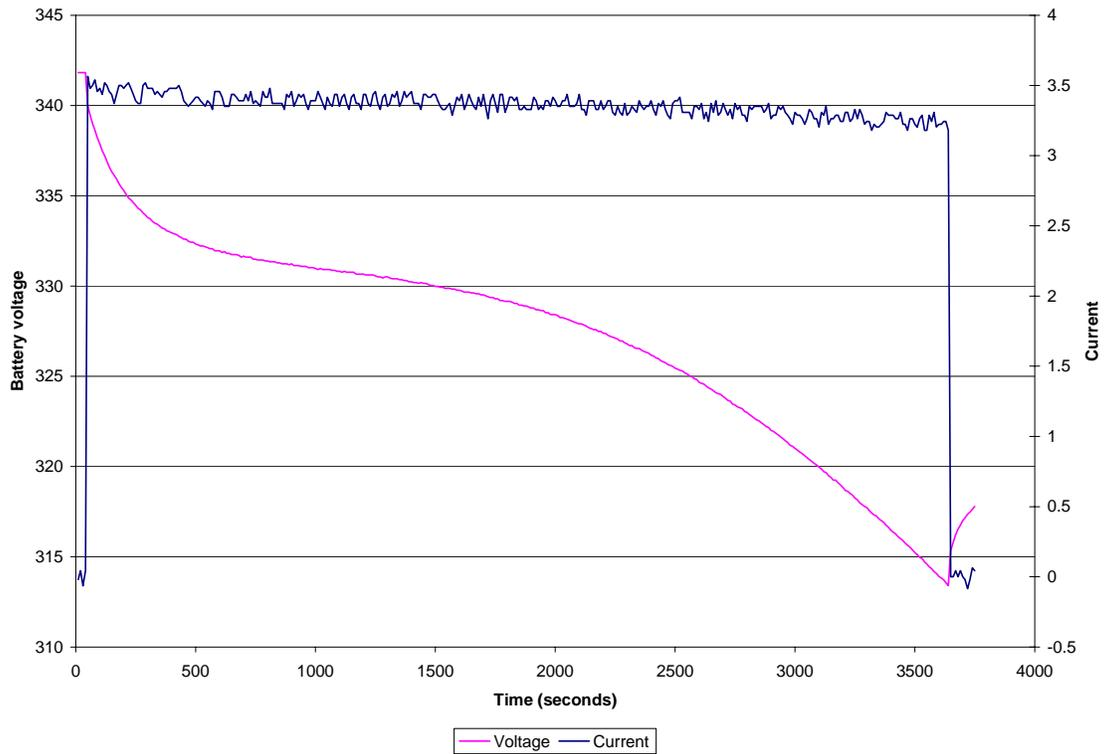
**Figure 39: Discharge at low current to 295V. Capacity removed = 0.79Ah**
