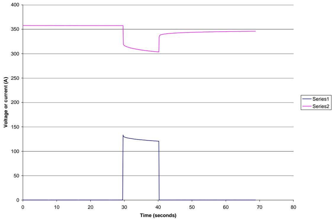
**Figure 62: Discharge at average current of 3.84A. Capacity = 4.38Ah**
