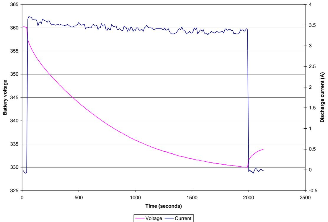
**Figure 47: Recharge at 2A following partial discharge. Charge input = 1.82Ah**
