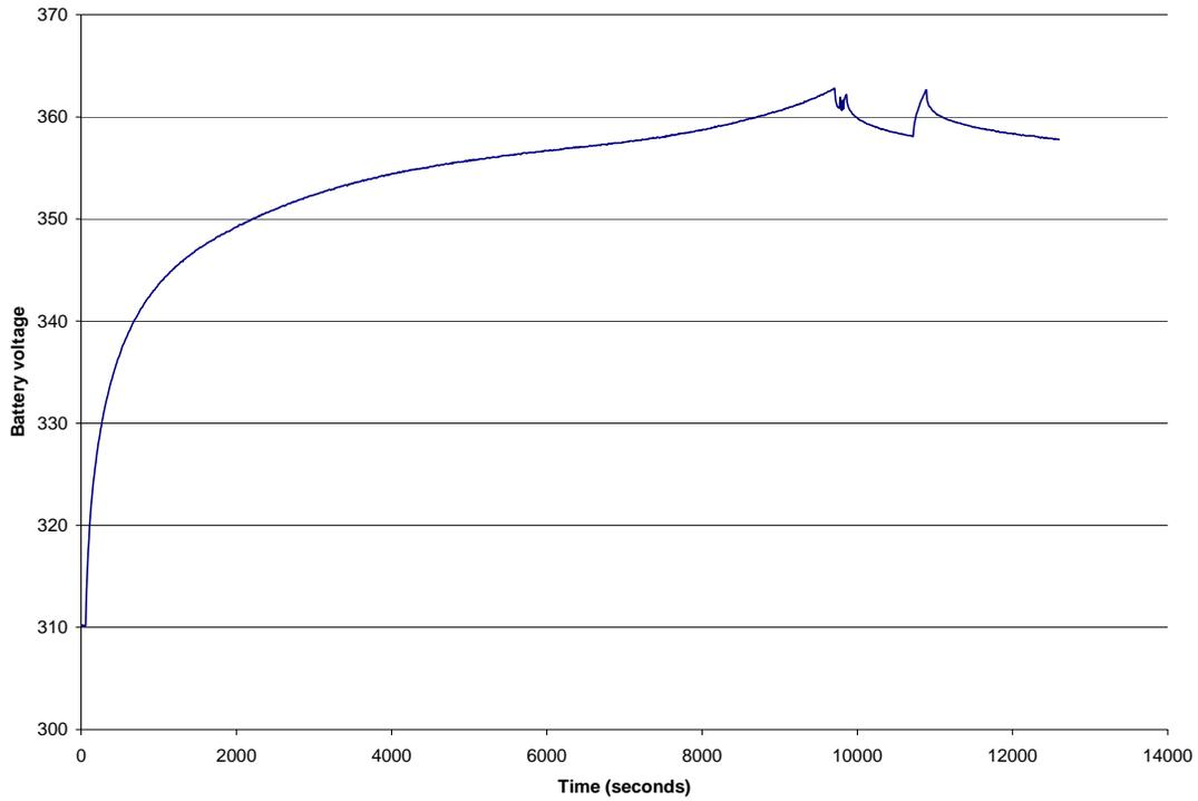
**Figure 36: First high current discharge (approx 65A) after full charge
