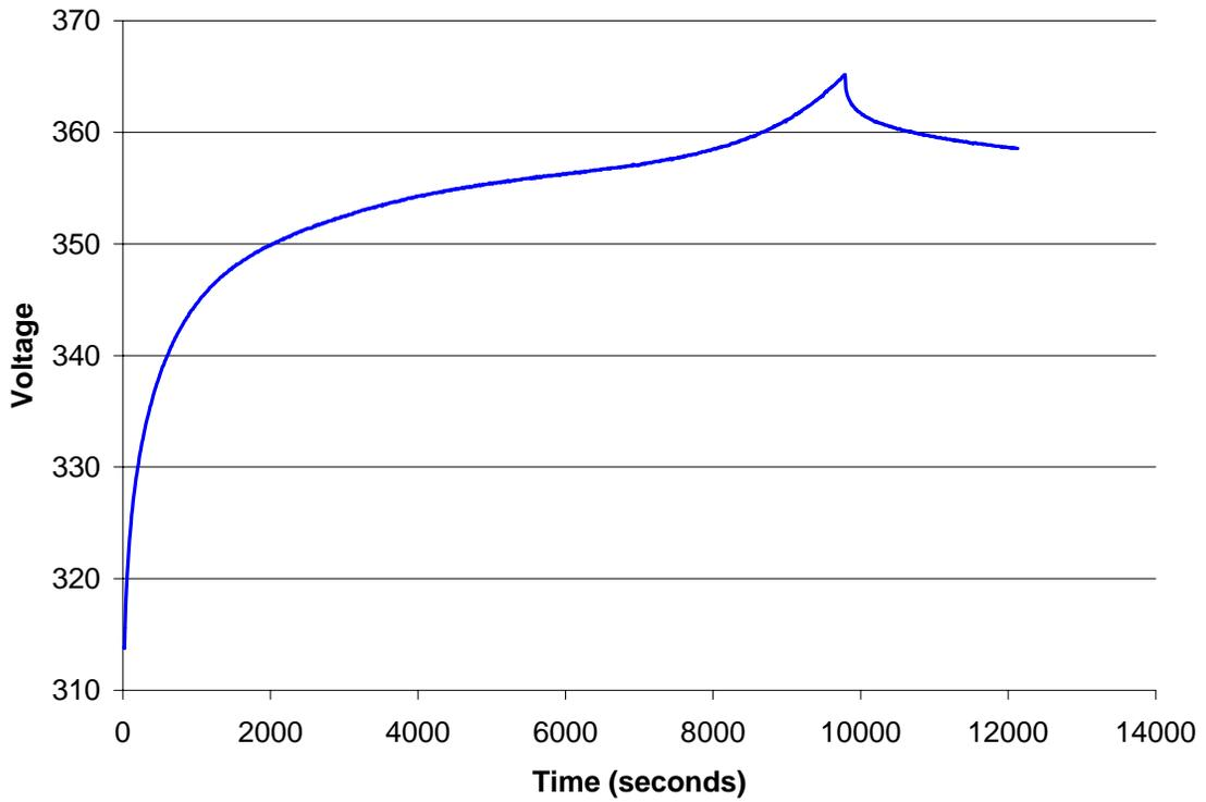
**Figure 54: High current discharge ( $I_{avg} = 77.2A$ ). Min voltage = 296.9V.
