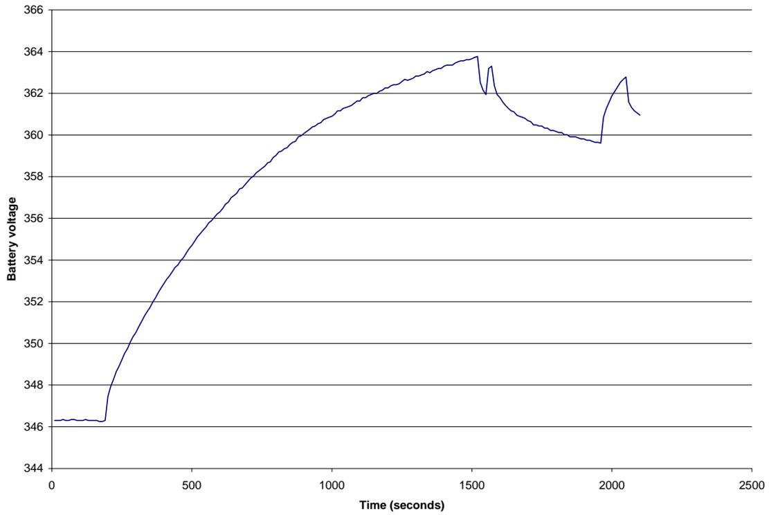
**Figure 46: Partial discharge at approx 3.5A. Capacity removed = 1.86Ah**
