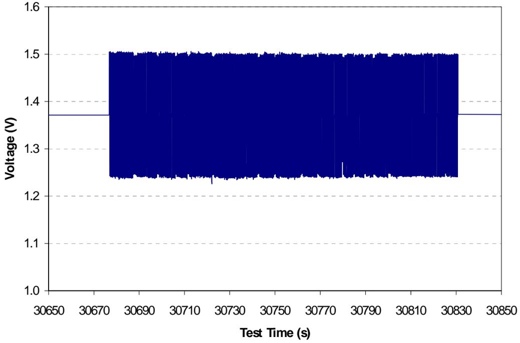
**Figure 10: Pulse cycling of cell S121-3 at 50% SOC**
