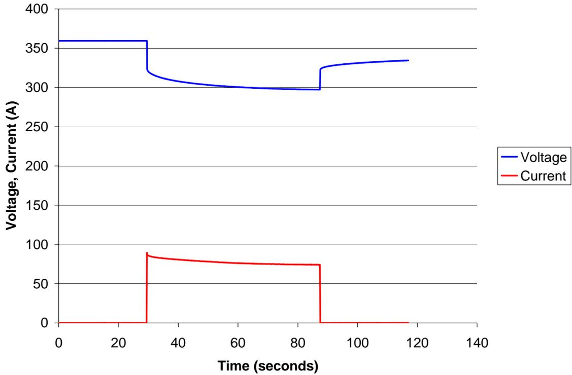
**Figure 51: Low current discharge ( $I_{avg} = 3.29A$ ). Capacity removed = 4.00Ah**
