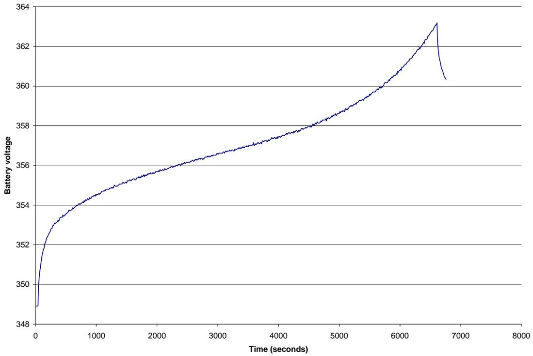
**Figure 42: Discharge at high current (approx 80A) for 1 minute. Capacity removed = 1.30Ah**
