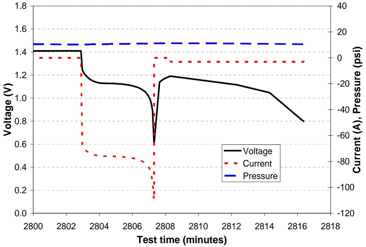
**Figure 19: Fast Charge Study Power and Energy Design Verification (PEDV) Test
