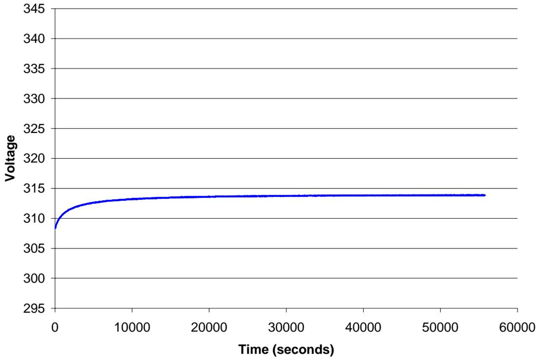
**Figure 53: Charge at 2.0A. Charge input = 5.40Ah**
