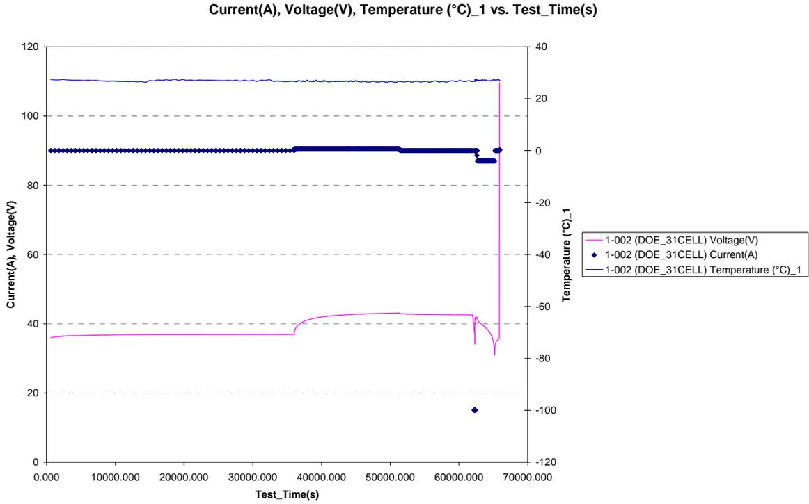
**Figure 23: 100A, 10 second discharge performed at 50% SOC**
