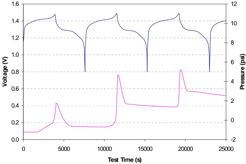
**Figure 8: Pulse discharge of S121-2**
