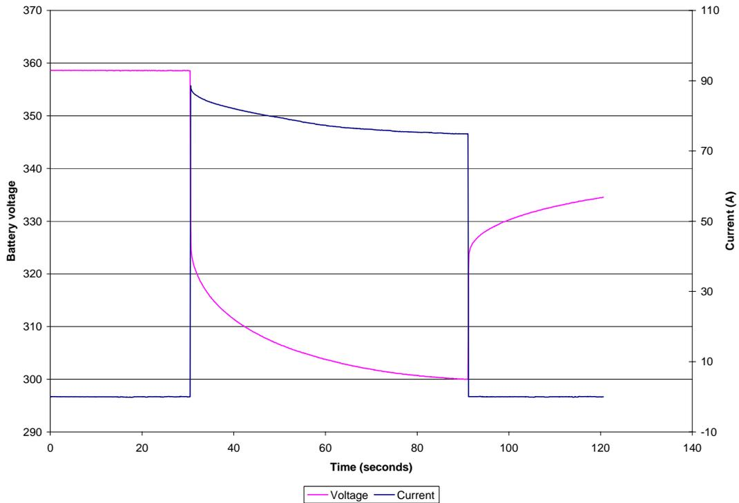
**Figure 43: Discharge at low current (approx 3.5A) to 295V.
