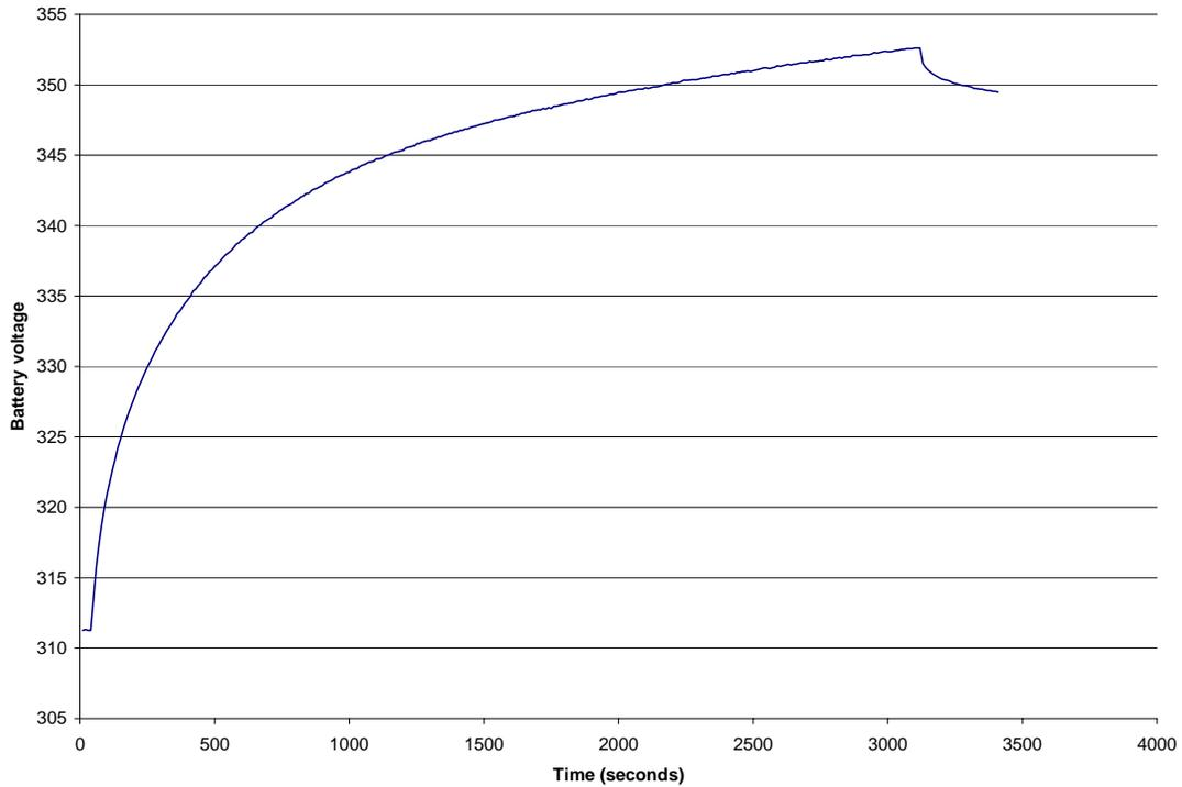
**Figure 41: Continuation of charge. Charge input = 3.65Ah**
