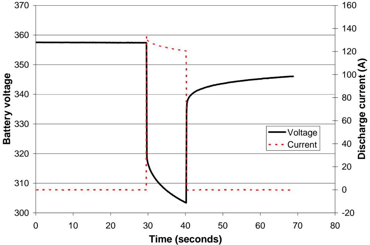
Figure 64: Customer-Generated Data 1 second 100A discharge
