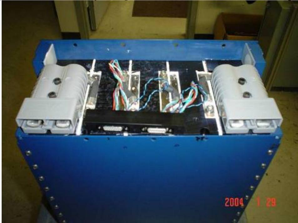
**Figure 34: 350V - Finished battery**
