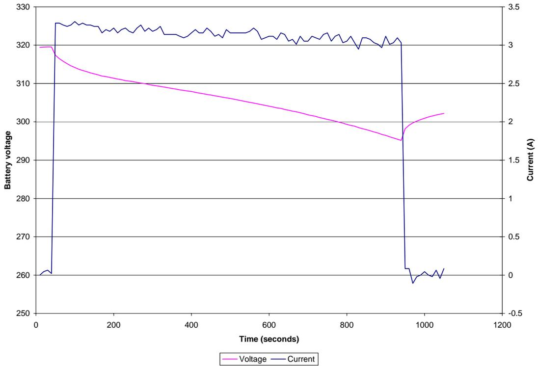
**Figure 40: Second charge at 2A. Capacity input = 1.71Ah.
