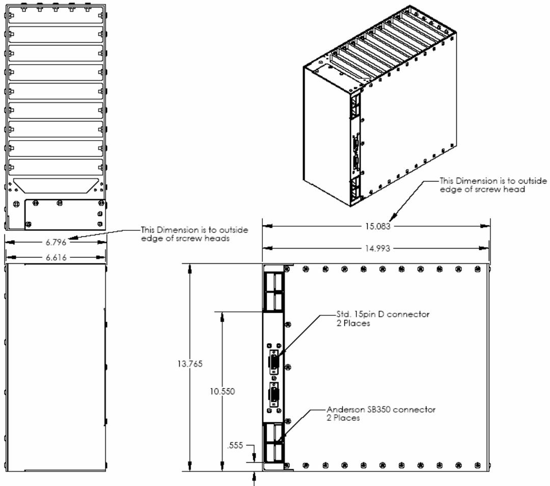
To get a better sense of the module design, it is instructive to examine the assembly sequence. First, each of the 5 packs is placed in the battery housing, which is shown in Figure 31. Before Compression, the total height of the assembly is greater than the internal space of the housing.
