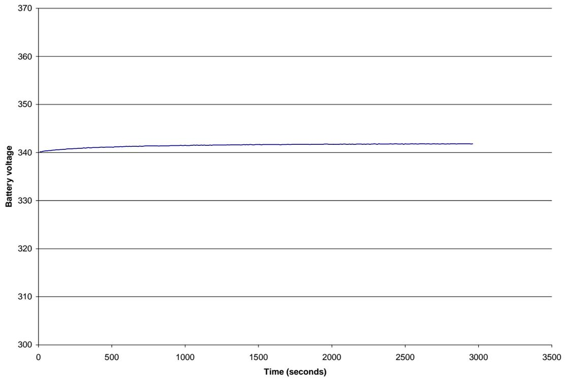
**Figure 38: Low current discharge (approx 3.5A) for 1 hour after rest
