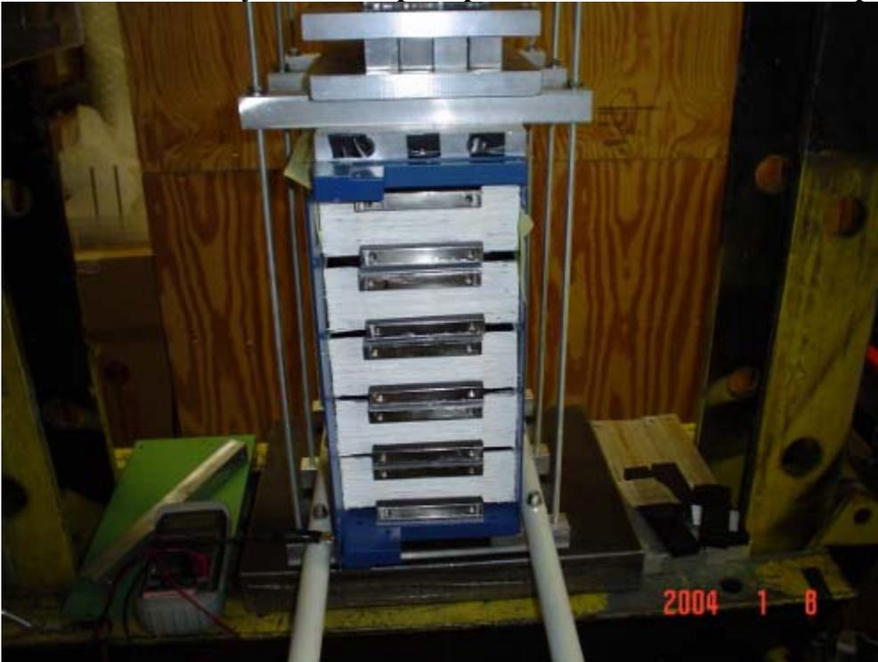
**Figure 33: 350V - Battery after power and sensor connections are completed**
