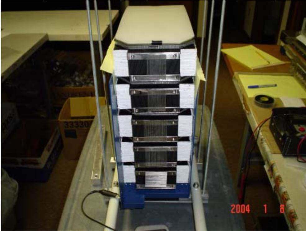
**Figure 32: 350V - battery after the top endplate has been installed and compressed**
