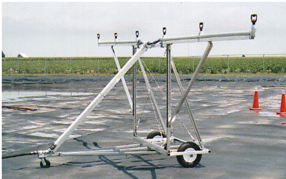
Figure 2 - Experimental Sprinkler Constructed by Argonne.
