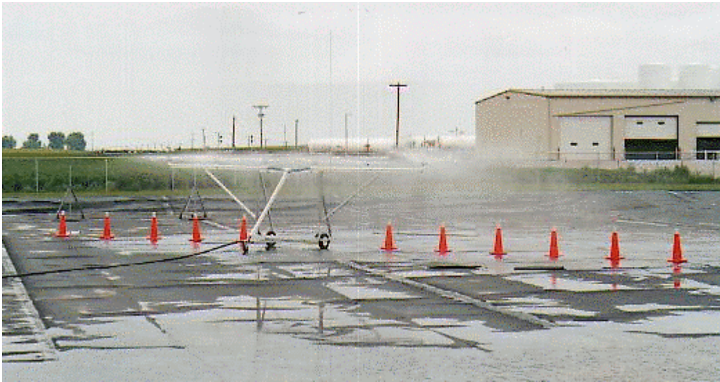
Figure 4 - Experimental Set-Up Used to Test the Performance of the Sprinkler.
