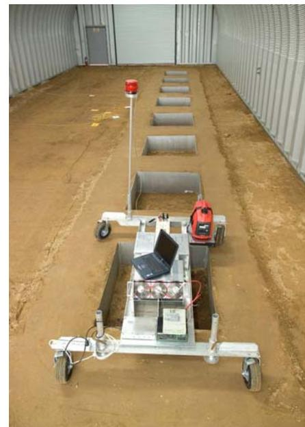
**Figure 4 A mobile INS system over a pit for synthetic soils.**
