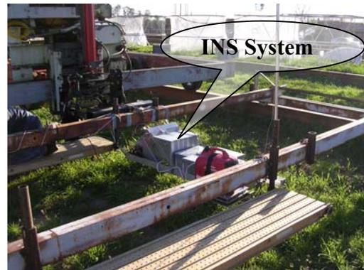
**Figure 2. INS system mounted on a scanning trolley**
