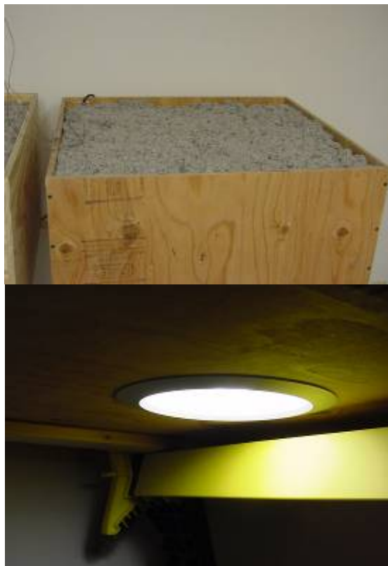
(b) Apparatus for recessed fixture
