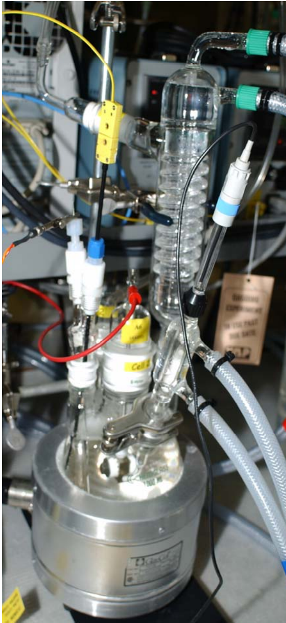
Figure 1 – Specimen and Experimental Apparatus for Electrochemical Testing
