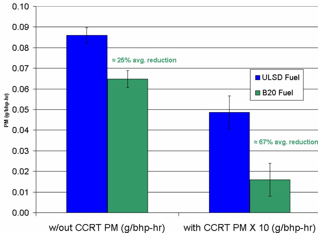
**Figure 6. Particulate matter emissions transient test results (error bars represent 95% confidence interval based on repeated tests)**
