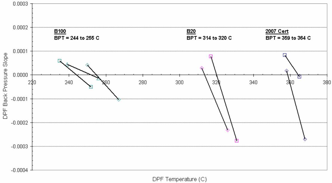
**Figure 3. BPT test results for B100, B20, and 2007 certification diesel**
