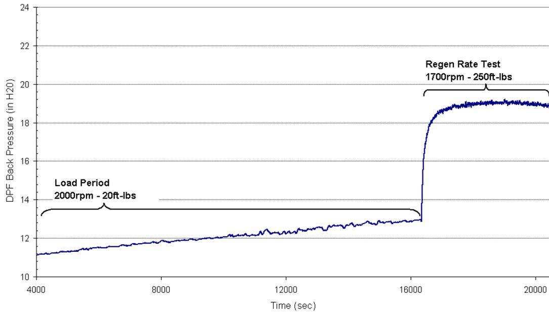
**Figure 4. Regeneration rate test DPF differential pressure**
