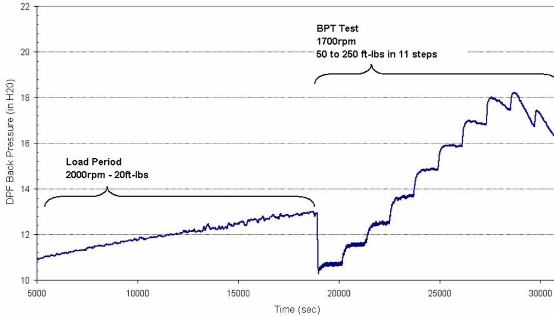
**Figure 2. DPF differential pressure during balance point temperature test**
