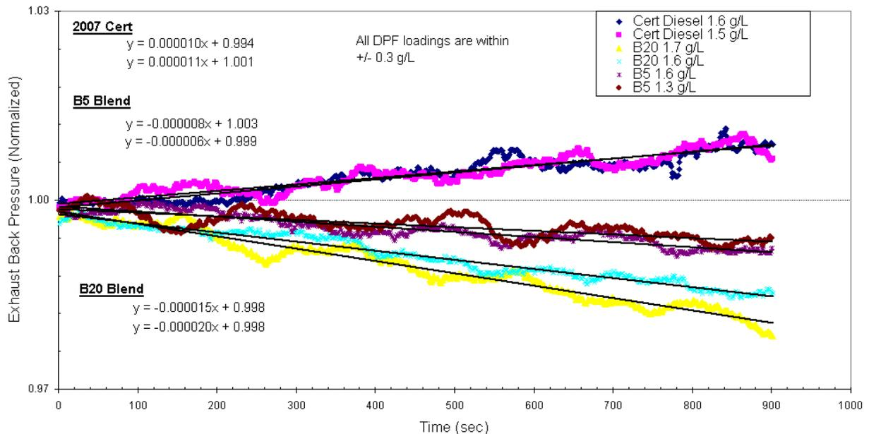
**Figure 5. Regeneration rate test results for B5, B20, and 2007 certification diesel**
