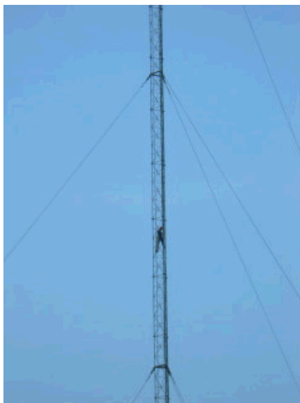
Fig. 3. Release of SF 6 from tower. Note man on tower controlling release valve.
