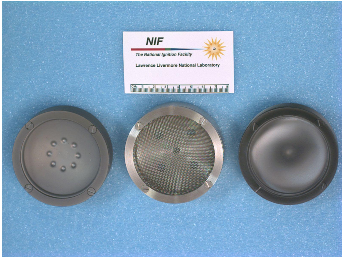
Figure 4. Bounce pans used for sputter coating. The pan on the left is used during the Be precoat, with up to eight capsules constrained to the dimples evident in the photo. The pan on the right is currently used when coating with up to twenty-four precoated capsules loaded. The pan the middle has a screen rather than a solid surface in order to allow debris to fall through rather than collect in the pan. All pans are mounted to a structure to minimize or eliminate resonance modes.
