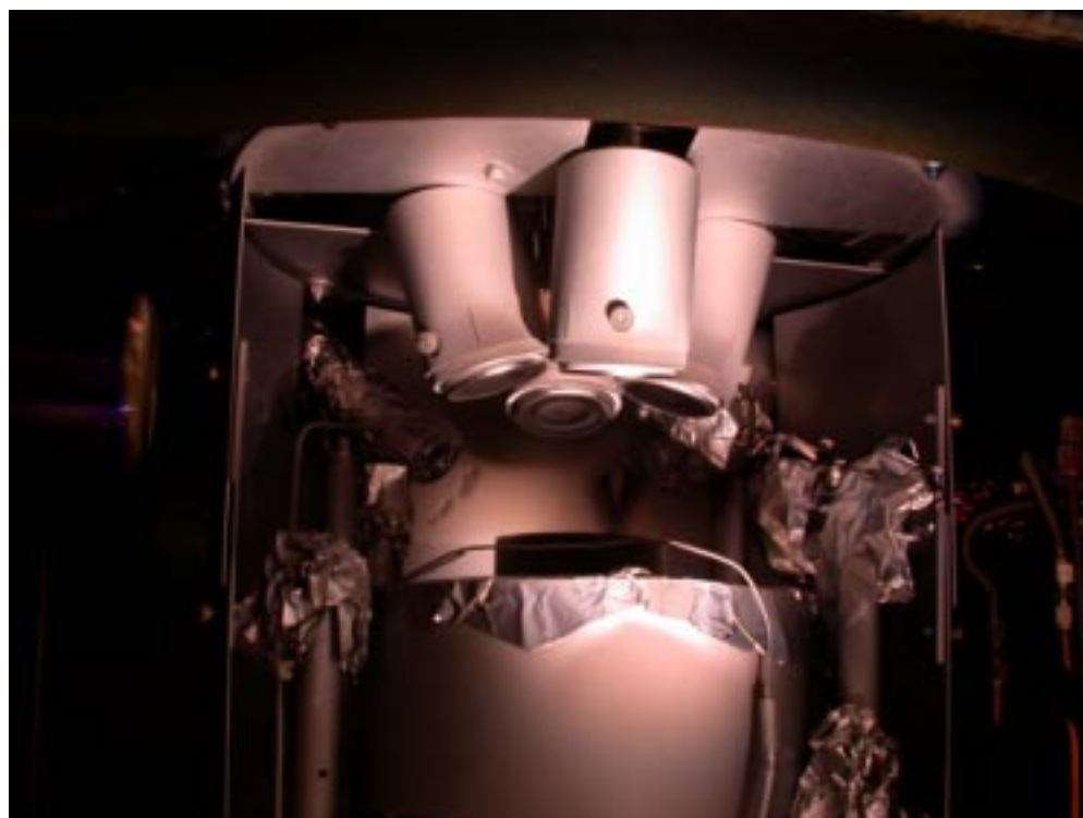
Figure 3. Photograph of the interior of the Be deposition system. The four Be guns are evident as well as the bounce pan.
