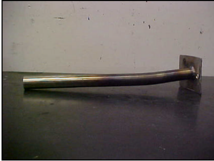
Figure 6. The initial design failed because the temperature was allowed to rise too quickly.
