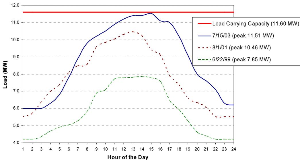
Figure 2. Hourly Load Profiles for Three Days with Broad Peaks.
