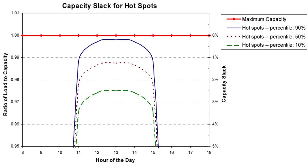
Figure 9. Variability of T&D Loading Relative to T&D Rating, Among Hot Spots.
