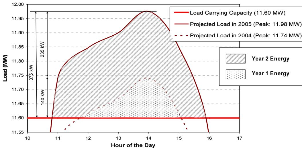
**Figure 8. Storage Power and Energy Requirements for Two Years of T&D Upgrade Deferral.**
