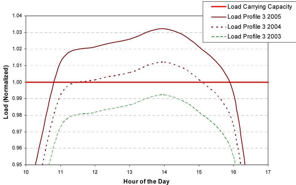
**Figure 5. Load Profile for Base Year and for two Subsequent Years, Reflecting a 2% Annual Load Growth Rate, and after Normalizing to the Annual Peak Load in the Base Year.**
