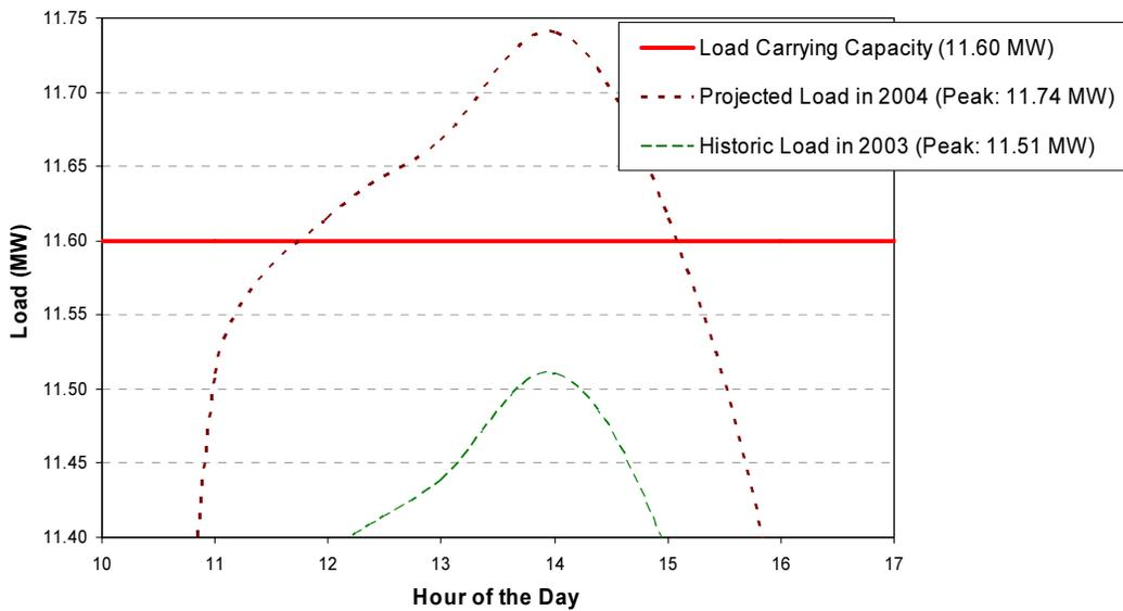
**Figure 6. Load Profiles for Base Year and after One Year of Projected Load Growth.**
