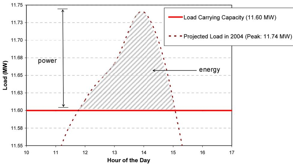
**Figure 7. Hourly Loads for Peak Day After Adding 2% to Reflect Load Growth.**
