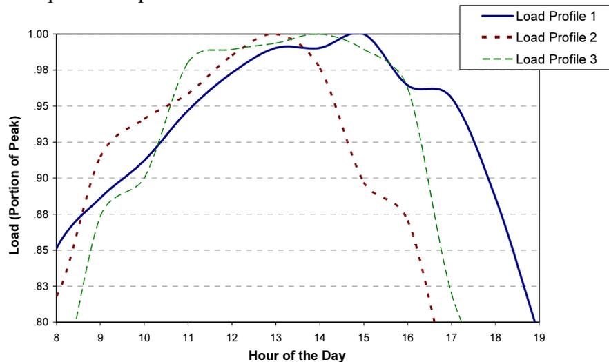
Figure 3. Normalized Hourly Load Profiles for Three Days with Broad Peaks Shown in Figure 2.
