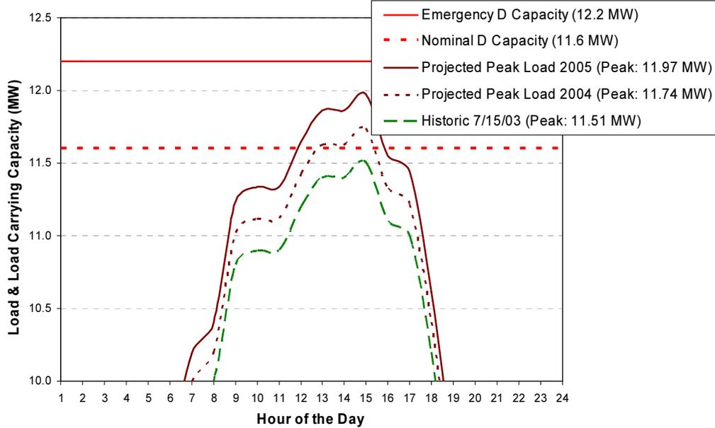
**Figure 1. Hourly Load for Highest Load Day in Summer, base Year Plus One and Plus Two Years of Projected Load Growth, Relative to Nominal and Emergency Distribution (D) Load Carrying Capacity.**
