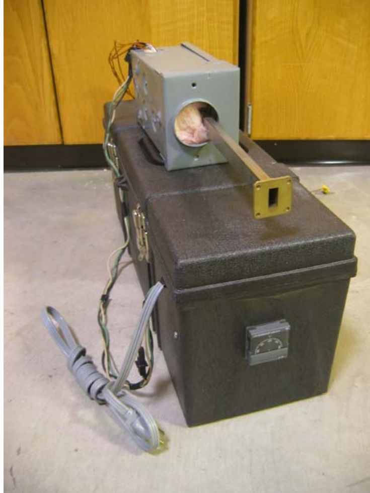
Fig. 1. Heated calibration load constructed for use with temperature measurement instrument. The microwave load is enclosed in heating tape inside the gray box. Control and power wires lead to the controller installed in the black box, which is also used as a carrying case. In operation, the microwave load temperature is controlled proportionally to within \pm 1 C of a desired setting.
