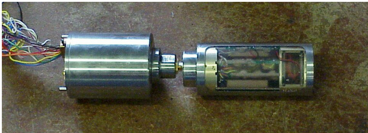
Figure 3-1: Photo showing the MDES unit (larger cylinder on the left) next to the MNVM/SiRES test unit (smaller unit on the right).
