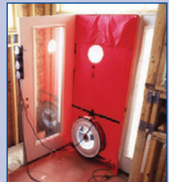
Home airtightness is tested with a blower door.
