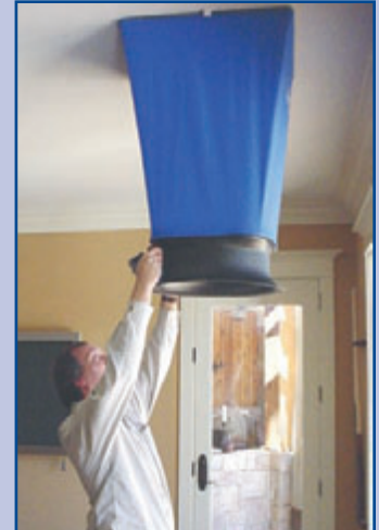
Air-flow testing ensures that the home's comfort meets the standards set during the design process.
