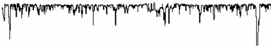
Figure 5-8: Typical plateau-honed finish
