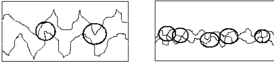
Figure 5-7: For rougher surfaces (left), fewer asperities contact than in smoother cases (right)
