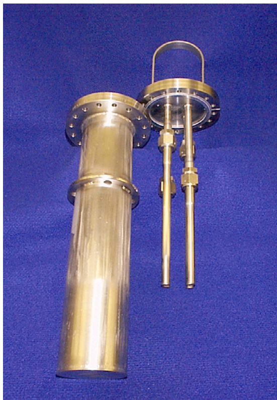
Fig. 3.7. Multiple-irradiation container used in HFIR SNF irradiations.
