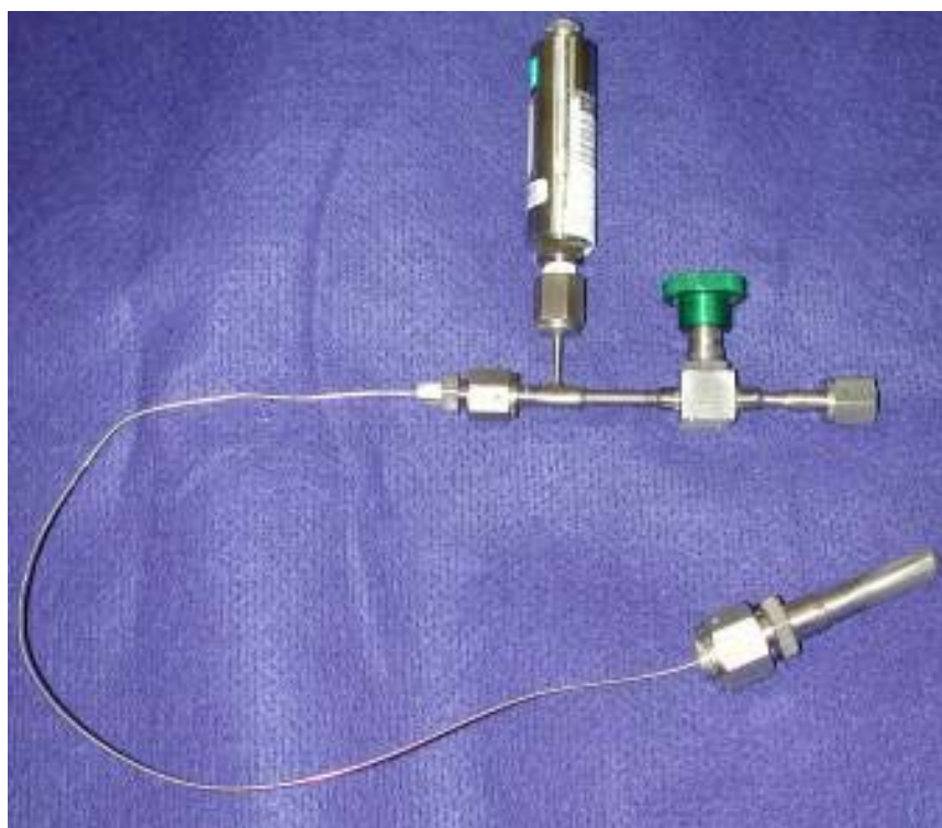
Fig. 3.9. Sample container and pressure transducer used in the alpha radiolysis experiments.
