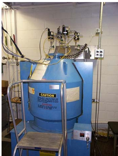
Fig. 3.1. ORNL ^{60}\text{Co} irradiator.
