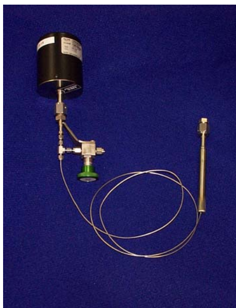
Fig. 3.2. Sample container and pressure transducer used in the ^{60}\text{Co} irradiations.
