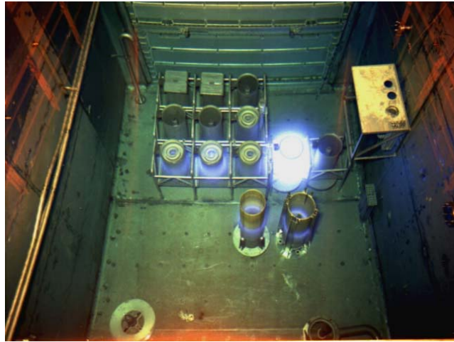
Fig. 3.5. SNF elements in the HFIR SNF pool.
