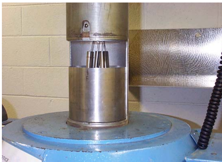
Fig. 3.3. Irradiation chamber of ORNL ^{60}\text{Co} irradiator with sample containers installed.
