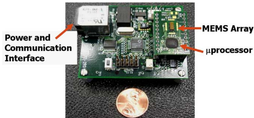
Figure 3. Integrated low-power, multisensor array
