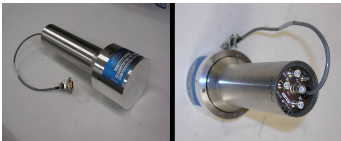
Fig. 5. FMFM gamma ray detector is composed of a commercially available BGO scintillation detector (left) and a preamplifier (right).
