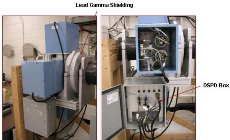
Fig. 12. View of the FMFM detector housing showing the detector interface electronics card (DIEC) and the sensor network communication (SNC) card.
