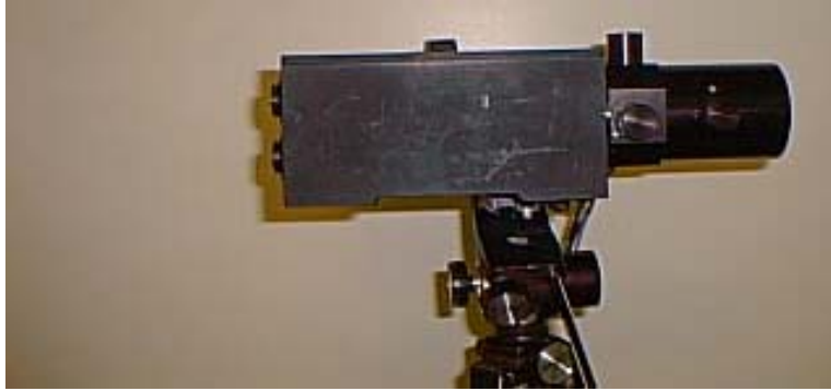
Figure 1. Photograph of the laboratory scale scanner mounted on a tripod.
