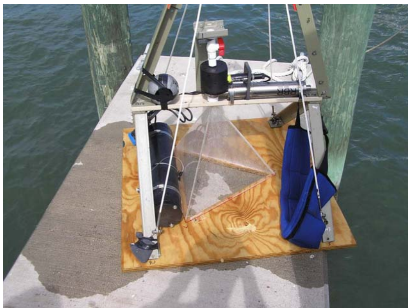
Figure 4. System configured for in situ testing, including funnel and pressure case.
