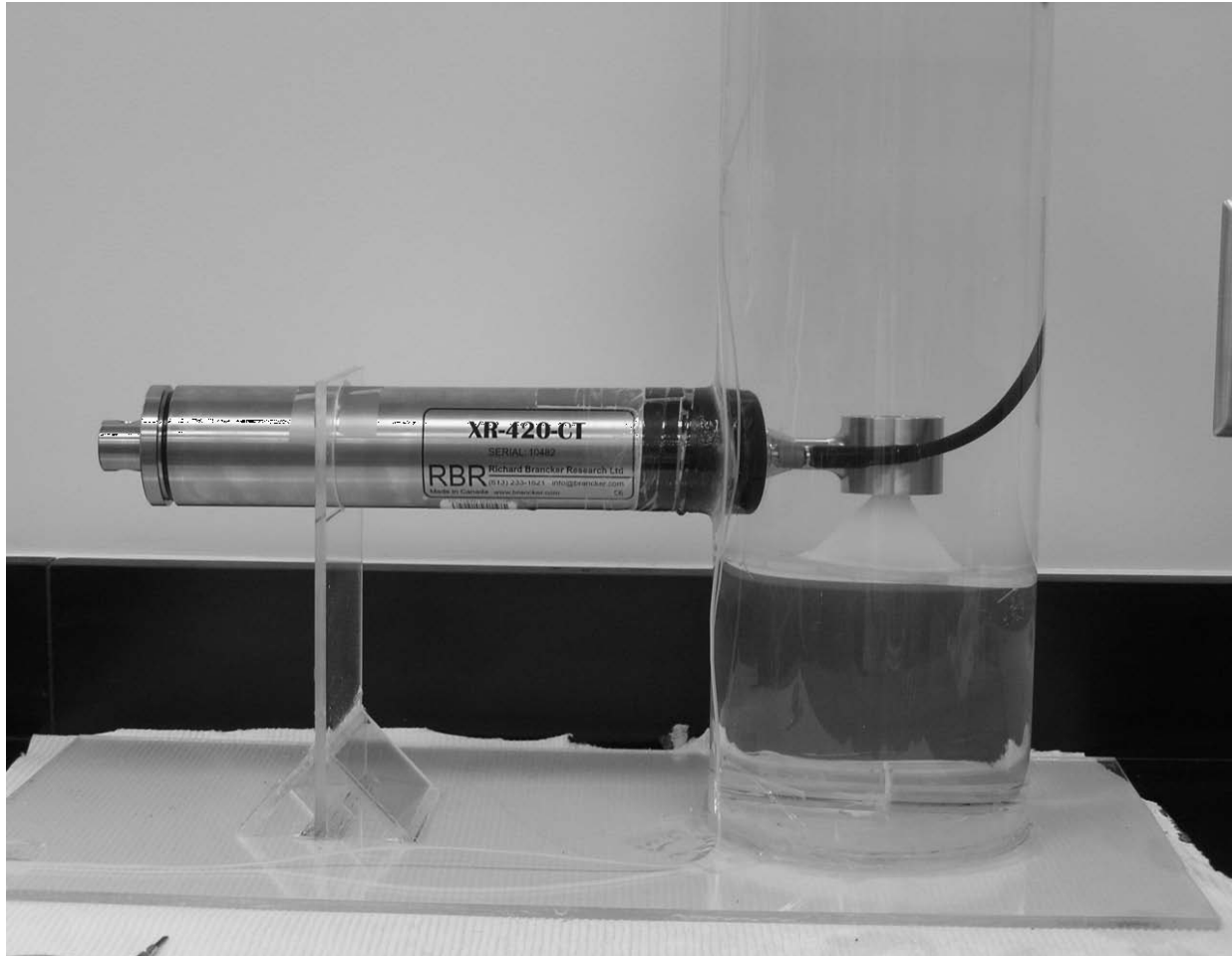
Figure 3. Laboratory test tank with Brancker conductivity sensor installed.
