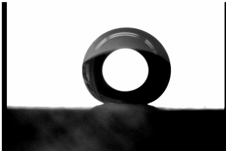
Figure 1: A drop of brine on a calcite plate treated with 0.2 wt% surfactant
