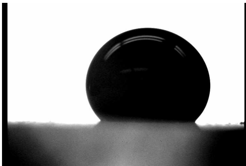
Figure 2: A drop of brine on a calcite plate treated with 0.2 wt% surfactant and aged in a field brine for 7 days
