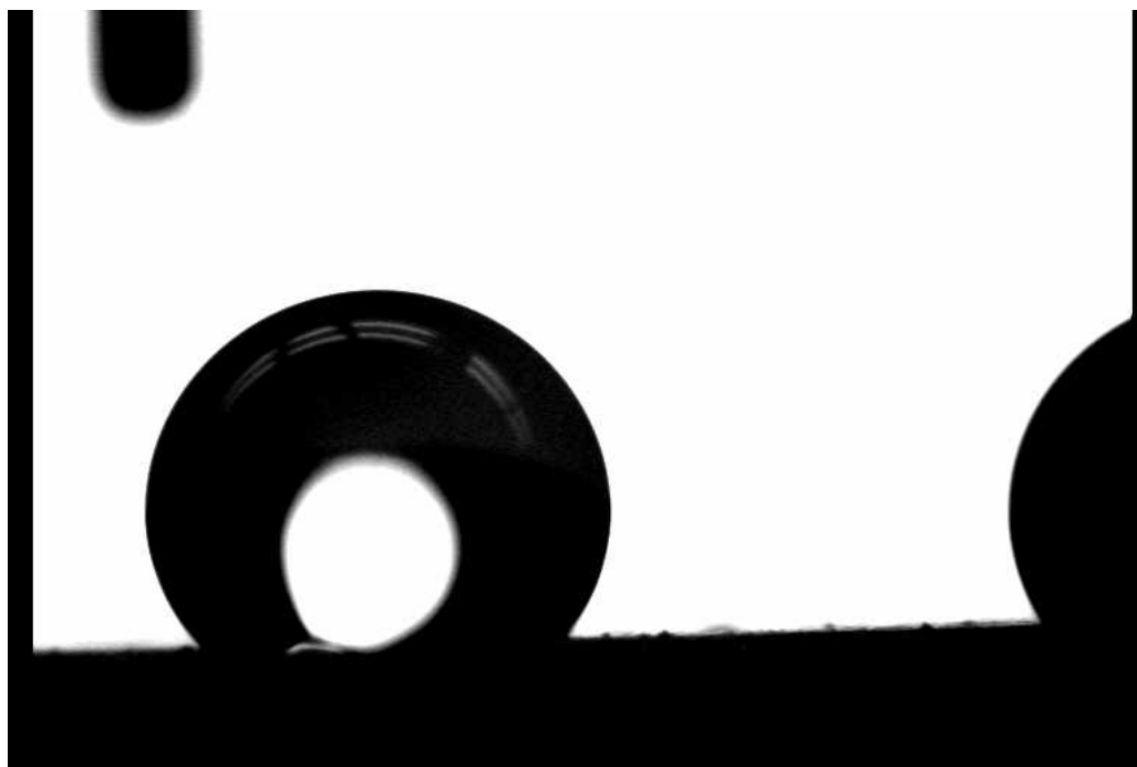
Figure 3: A drop of decane (surrounded by air) on a calcite plate treated with the surfactant
