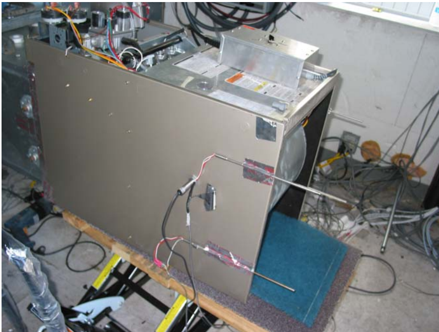
Figure 13. Furnace mounted in electric utility test apparatus
