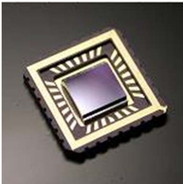
Figure 39 MEMS chip in wafer level package attached to LCC (only for electrical connections in test).
